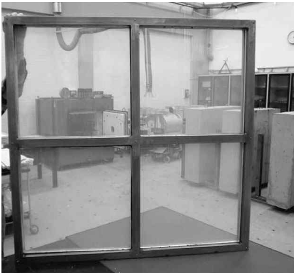
10.4 An aerogel window manufactured by joining four optimized aerogel tile prototypes in a test frame (Jensen et al. , 2004).
