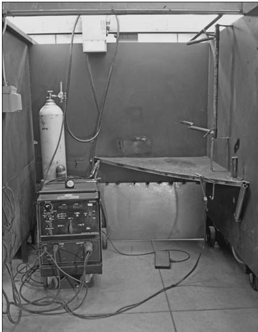
Figure 7-1: A tig welding setup.
