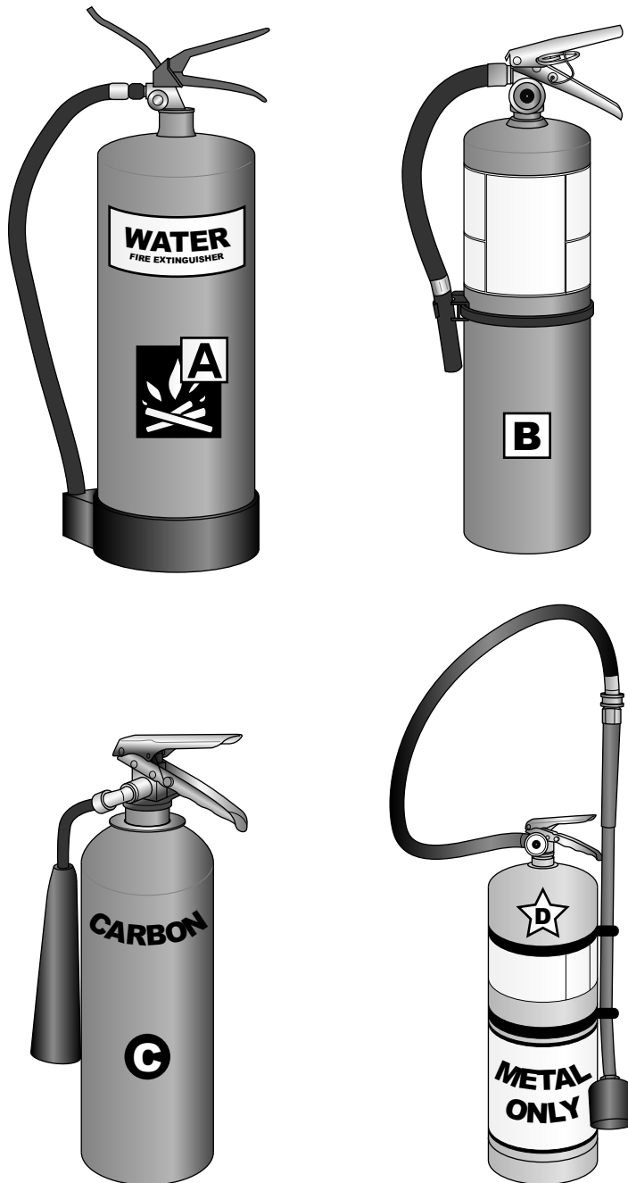
Figure 3-2: Four classes of fire extin- guishers.
