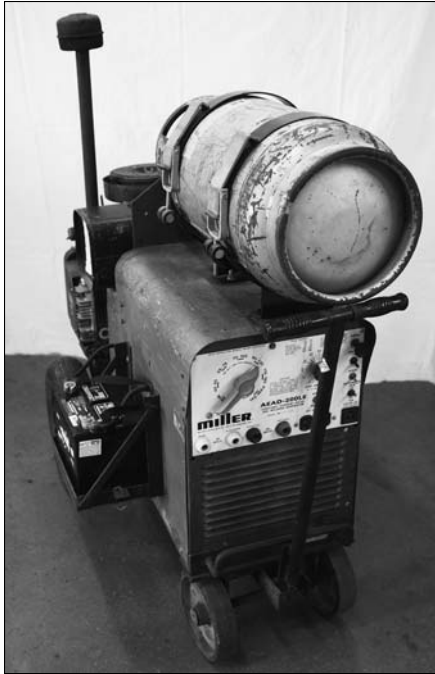
Figure 5-1: A generator stick welding machine.
