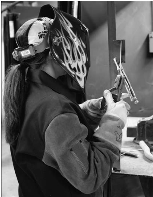
Figure 6-6: Practicing vertical- down stick welding.
