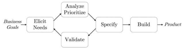
Figure 3.3 Requirements development is completed before the build phase, during plan-driven development. This diagram adds a specify activity between analyze and validate in Fig. 3.1 .
