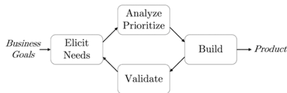
Figure 3.2 Requirements development is an integral part of agile software development. This diagram adds a build activity between analyze and validate in Fig. 3.1 .
