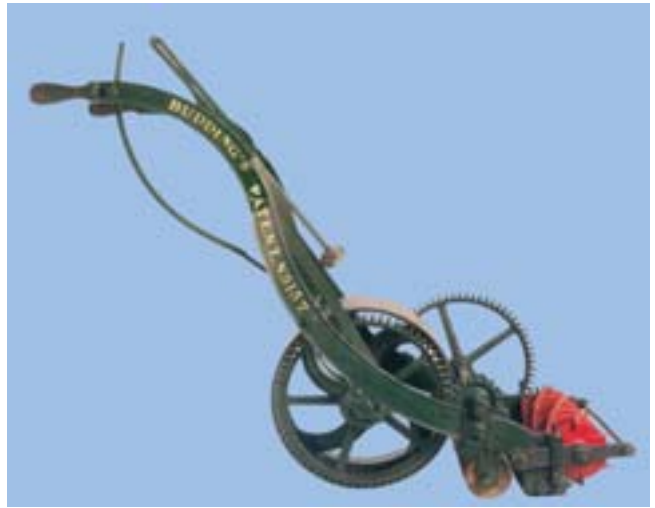
Lawn-mover is a combination of kinematic links.
