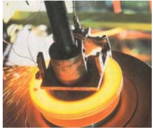
In a disc brake, hydraulic pressure forces friction pads to squeeze a metal disc that rotates on the same axle as the wheel. Here a disc brake is being tested.
