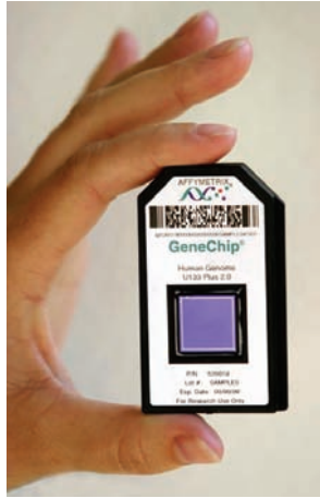
FIGURE 2.1: Image of a standard Affymetrix microarray. On a surface of 1.3 cm x 1.3 cm millions of probes with different sequences are present to quantify the abundance of all mRNA species incoded by the human genome. Image courtesy of Affymetrix.
