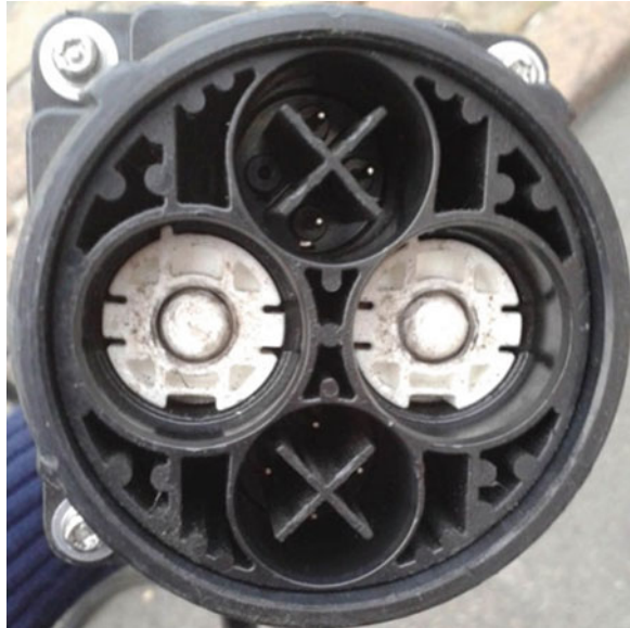
Fig. 3 Yazaki (CHAdeMO) plug (vehicle connector)
