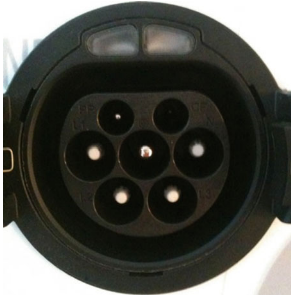
Fig. 2 Type 2 socket (vehicle inlet)
