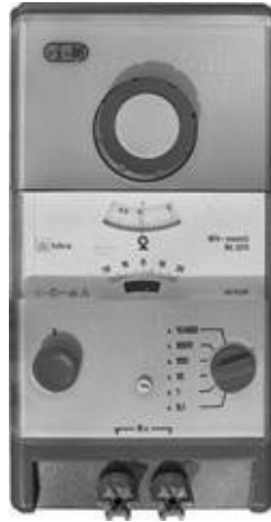
Figure 5.3 Commercial Wheatstone bridge
