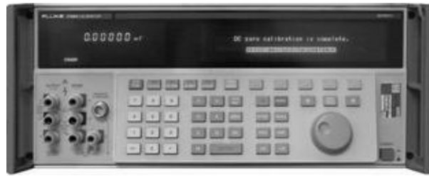
Figure 5.11 Precise DC voltage calibrator Fluke 5500 in the Primary Electromagnetic Laboratory of Croatia
