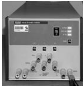
Figure 3.27 Zener voltage standard at the Croatian Primary Electromagnetic Laboratory
