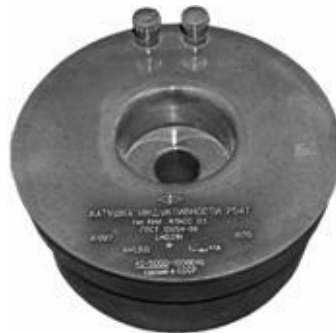
Figure 3.21 Inductance standard of 0.01 H
