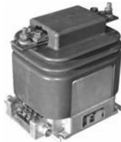
Figure 6.11 Current transformer at the Faculty of Electrical Engineering and Computing in Zagreb
