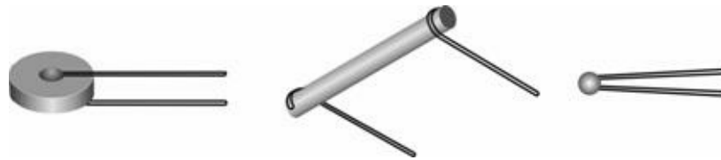
Figure 12.7 Types of thermistors
