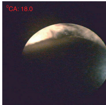
Figure 27. Moment of ignition took place for 10 deg CA before TDC. The photograph present the initial phase of flame development for 18 deg CA after TDC. High whirling occurring in the combustion chamber is clearly visible.
