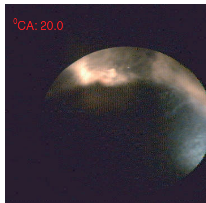
Figure 28. Photograph of the further development of the flame for 20 deg CA after TDC. The flame spreads over the whole combustion chamber and the flame front moves towards the zone of expression
