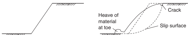
Fig. 13.5 Typical rotational slip in a cohesive soil.
