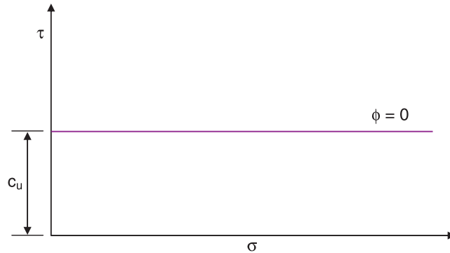
Fig. 4.9 A cohesive soil, subjected to undrained conditions and zero total normal stress will still exhibit a shear stress, c_u .
