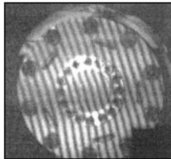
Figure 7 – Parallel fringes on front flange indicate no vibration.
