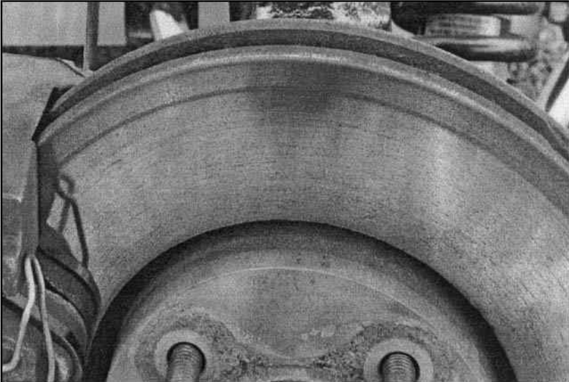
Figure 7c: Condition of coating “A” on outer surface of front offside disc of Cosworth powered Dax Rush hill climb car after a full racing season.
