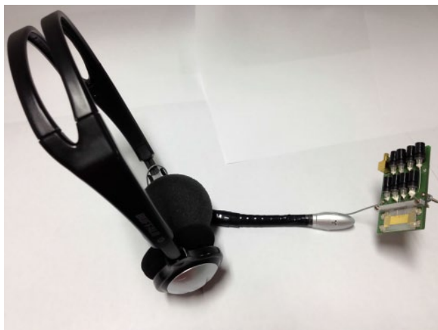
Figure 7.18 Photo of olfactory display using eight EO pumps and SAW device
