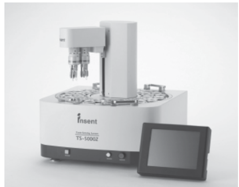
Figure 4.4 Models of the taste sensing system. (a) First model: SA401; (b) second model: SA402; (c) third model: SA402B; and (d) fourth model: TS-5000Z. Republished with permission from Ref. [124]. Copyright 2013, Pan Stanford Publishing
