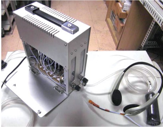
Figure 7.17 Compact olfactory display using 13 components (available from Ono Denki Inc.)
