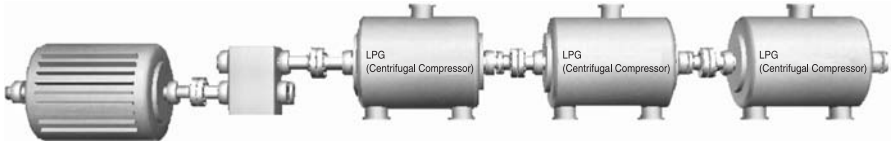
Figure 2-1 Turbomachines connected by shaft couplings. Courtesy of GE Energy.*
