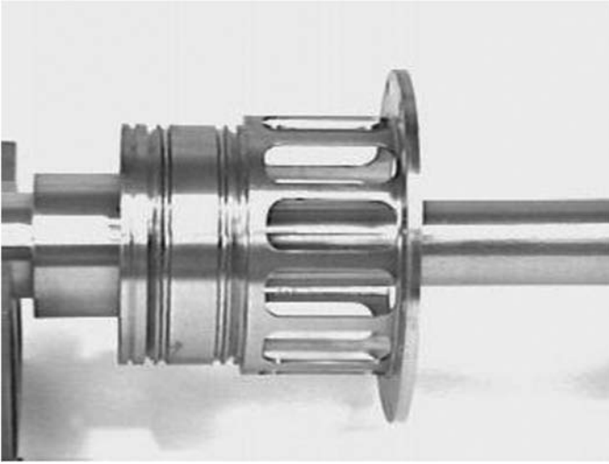
Figure 5-56 Actual squirrel cage damper with the damper journal on the left end.
