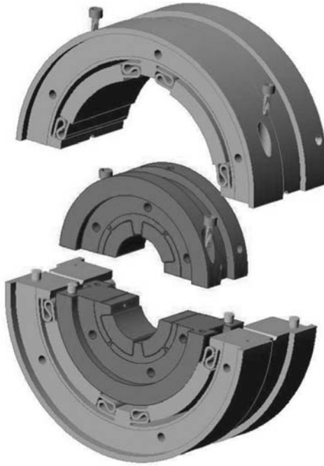
Figure 5-57 Schematic of original integral squeeze film damper.
