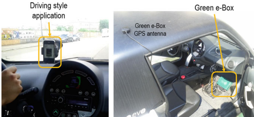
Fig. 8 Test vehicle: the iPhone with the driving style application ( left ) and the electronic control unit, Green e-Box ( right )
