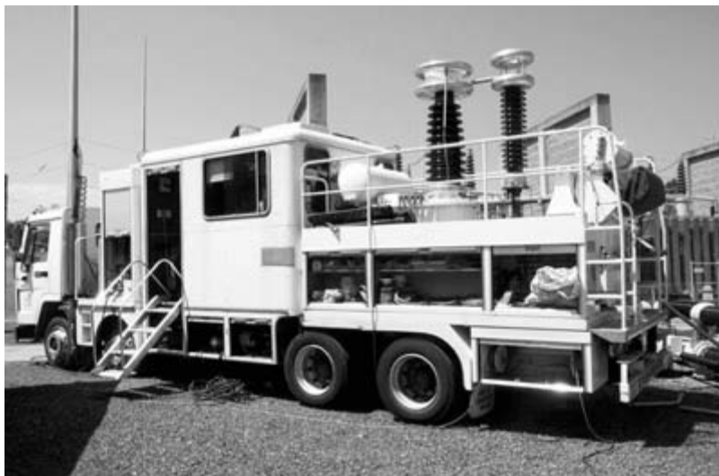
Figure 6.9 Example of high-voltage test vehicle (250 kV testing transformer and ancillary equipment) [photograph by Enerserve (Energy Australia)]
