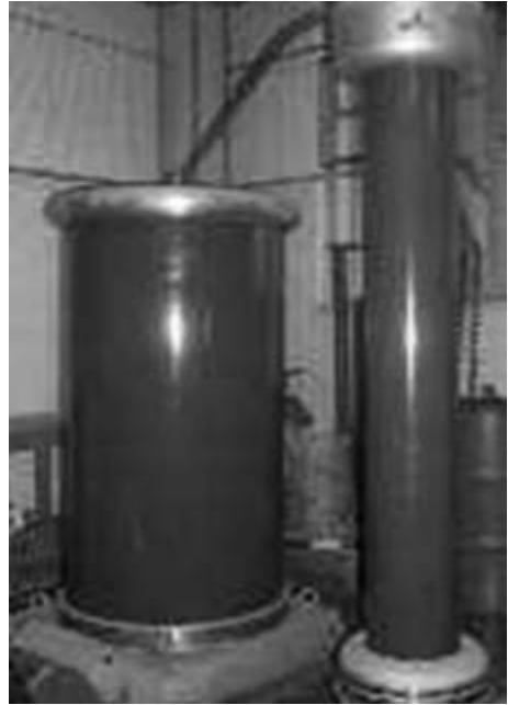
Figure 6.2 250 kV testing transformer and capacitor divider – insulation cylinders as shells
