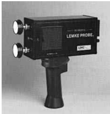
Figure 8.3 A portable PD detector with exchangeable capacitive and inductive sensors [courtesy of Lemke Diagnostics AG, URL: http://www.ldic.ch , http://www.hvdiagnostics.de ]
