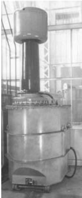
Figure 6.1 200 kV testing transformer – metal tank
