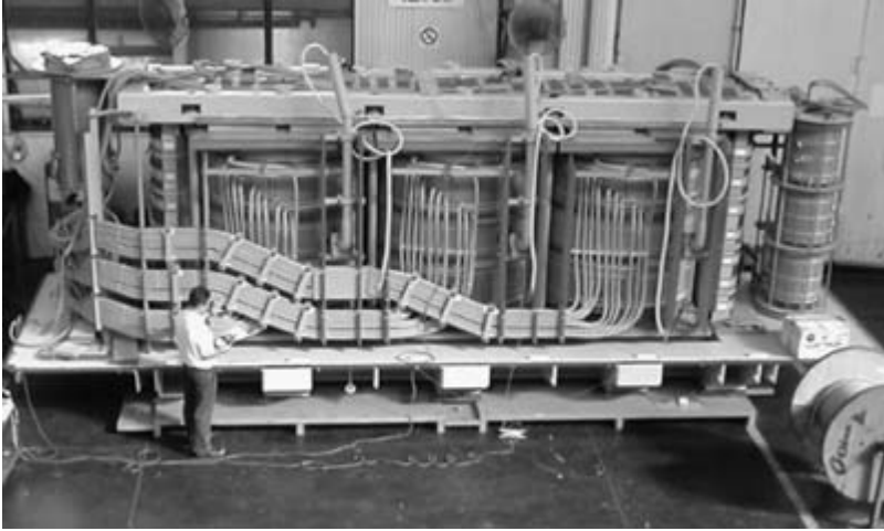
Figure 5.8 Core and coils of a 225 MVA, 220/66/11 kV substation transformer with outside taps and centre-entry high-voltage leads [photograph by AREVA T&D, Brisbane, Australia]
