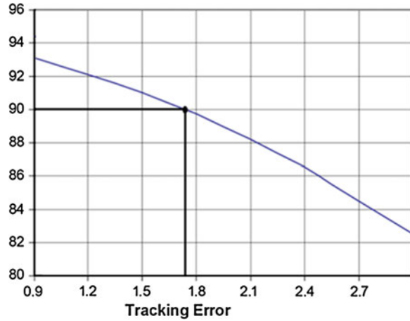
Fig. 5 Example of the variation of the module power (%) versus tracking error ( ^{\circ} ). In this case, the acceptance angle is 1.7^{\circ}
