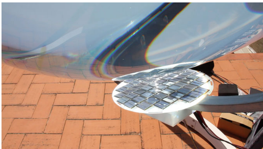
Fig. 14 Photograph of the receptor formed by a matrix of cells. Courtesy of Rawlemon
