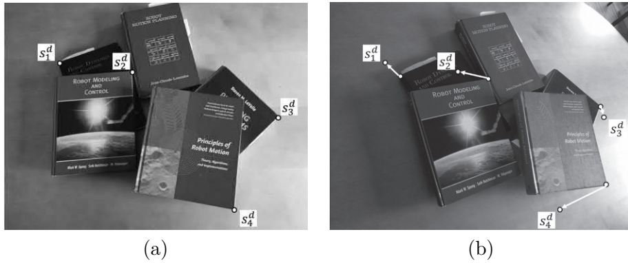
Figure 11.6: The goal image is shown on the left. When the camera reaches the desired configuration, the features s_1^d, s_2^d, s_3^d, s_4^d will be located as shown in this image. The initial image is shown on the right, along with four error vectors that correspond to the four image features.
