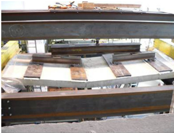
Figure 5.18 Full-scale specimens of posttensioned concrete slabs tested and modeled by Ellobody and Bailey [5.4].
