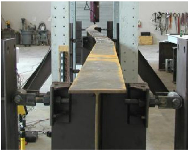
Figure 6.20 Comparison of experimental and numerical deformed shapes at failure of the full-scale built-up I-section plate girder T3.
