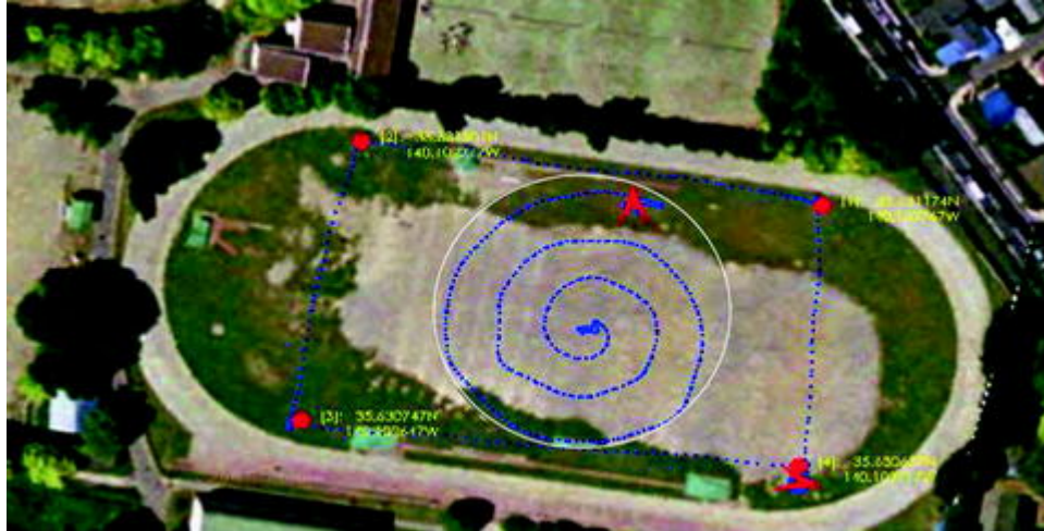
Fig. 8.10 Part of the GCS interface showing a 2D map of test field and MAV trajectories during waypoint navigation and spiral trajectory tracking
