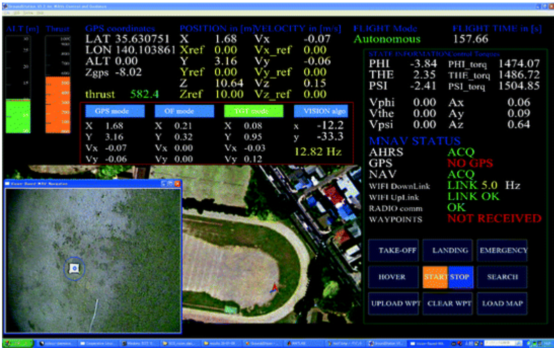
Fig. 12.6 The interactive interface of the ground control station during vision-based autonomous hovering
