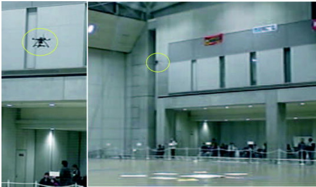
Fig. 10.6 The quadrotor UAV in autonomous indoor flight using optic flow
