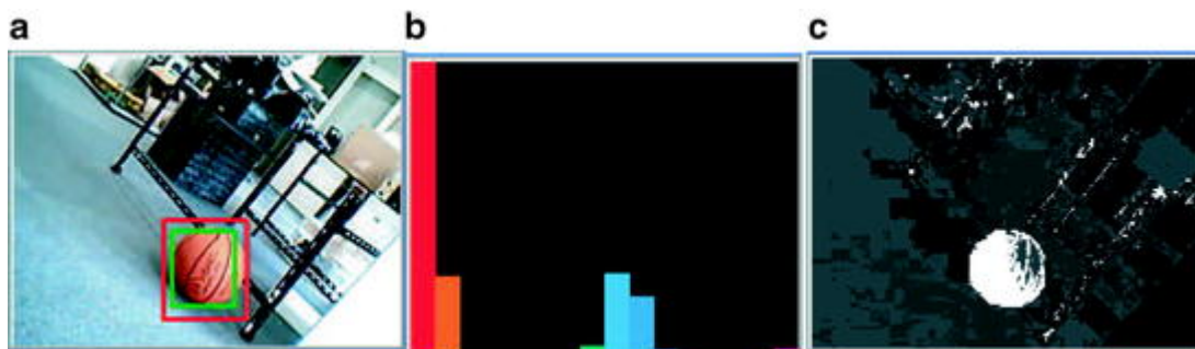
Fig. 10.10 (a) Result of the tracking, after rotating the camera, (b) Color histogram of the ball, (c) The backprojected image based on color probability distribution
