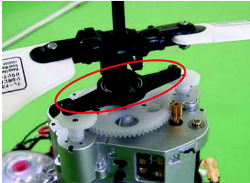
Fig. 2.4 Swash plate of coaxial-rotor helicopter
