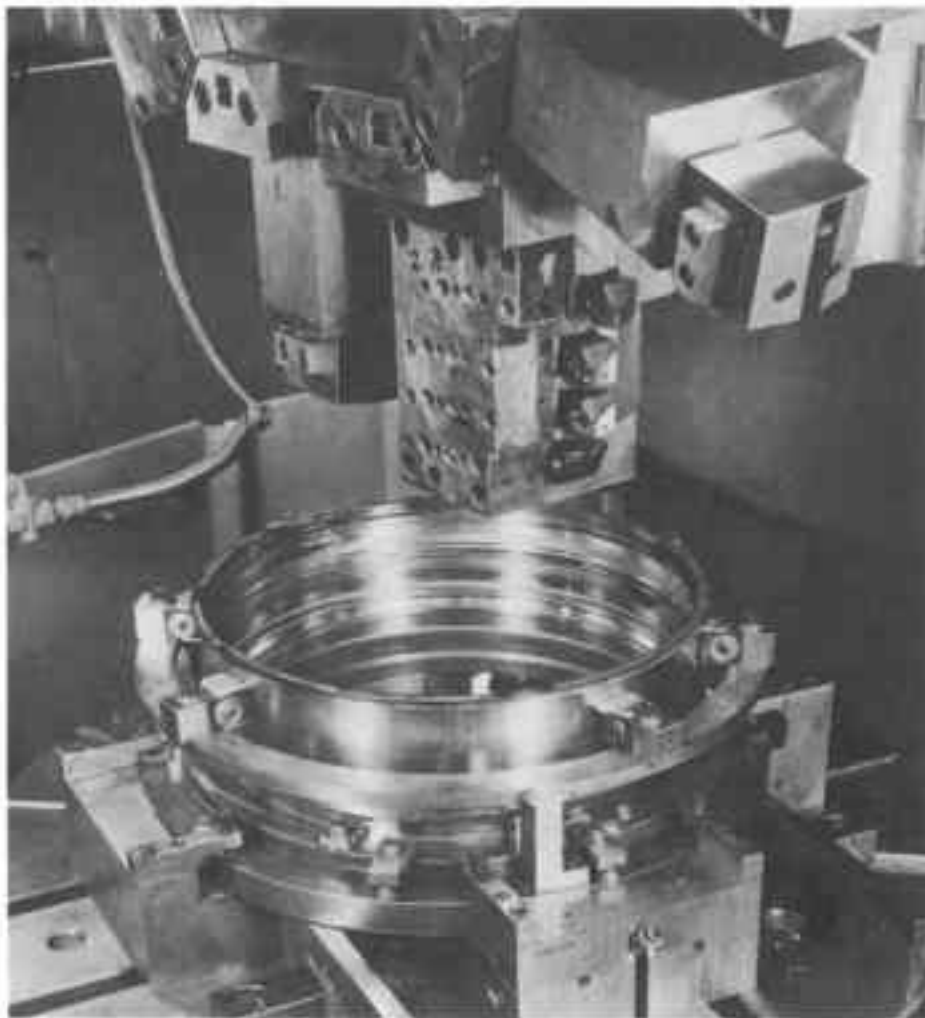
Fig. 14-27. Special work-holding fixture and tooling blocks on vertical turret lathe.
