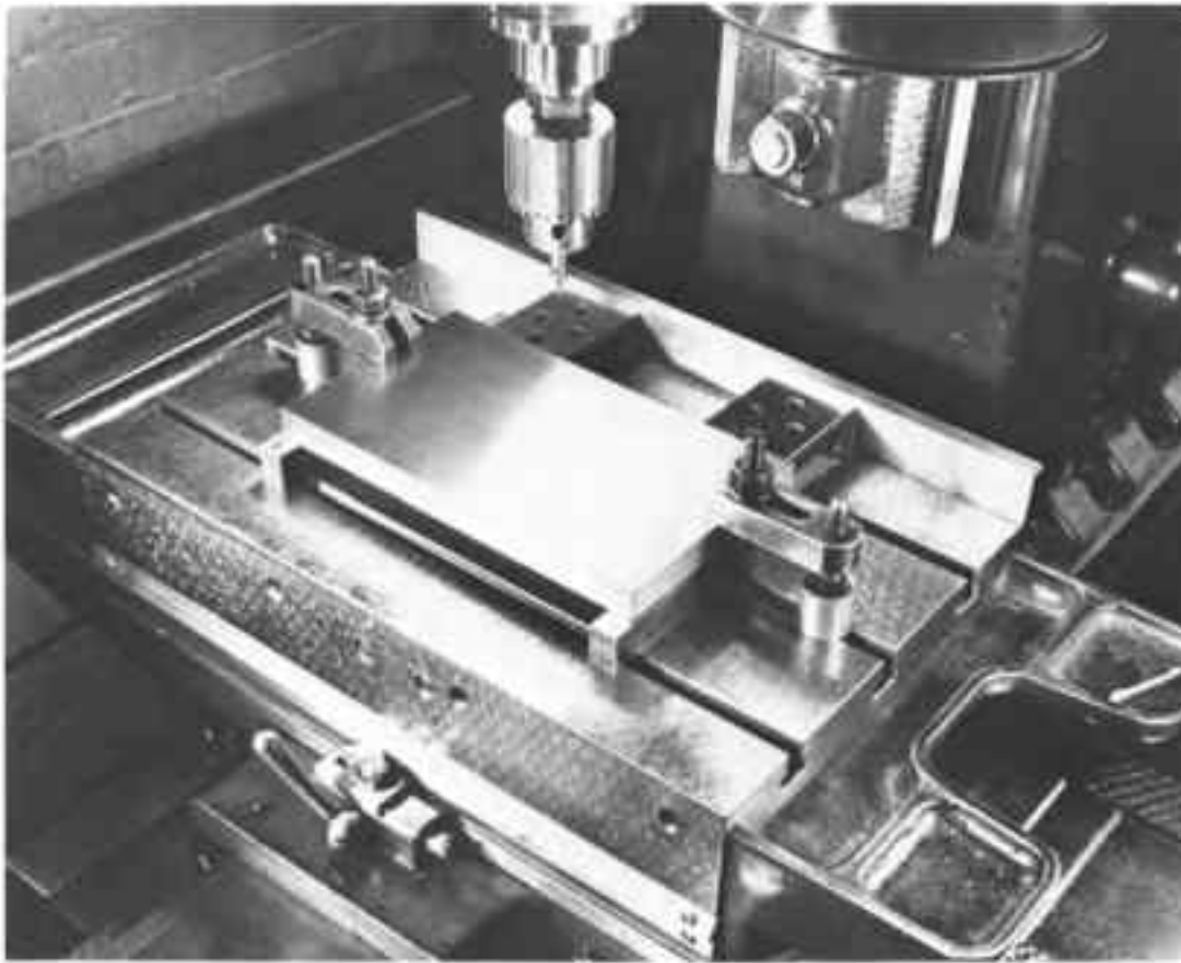
Fig. 15-19. Using straightedge attached to table and precision setup blocks to align workpiece parallel to the table travel.
