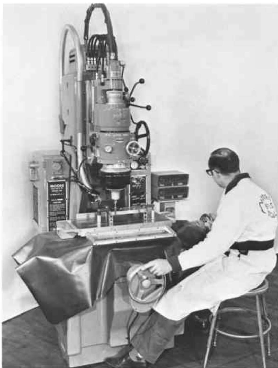
Fig. 15-40. Precision jig-grinder with switchable inch-metric digital readout. Positioning accuracy is .000030 inch in one inch and .000000 inch in 18 inches.
