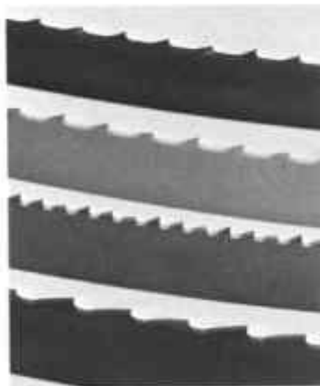
Fig. 16-8. The basic band-saw blade-tooth forms. The names of the tooth forms from top to bottom are: butress, claw tooth, precision, and tungsten carbide.
