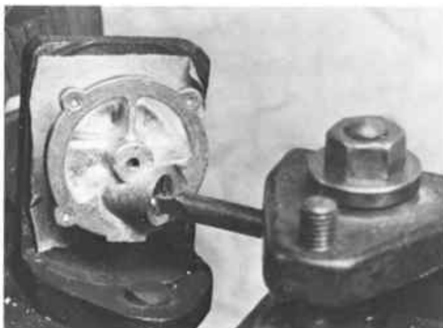
Fig. 11-19. Using two angle plates mounted on a faceplate to hold a small casting.
