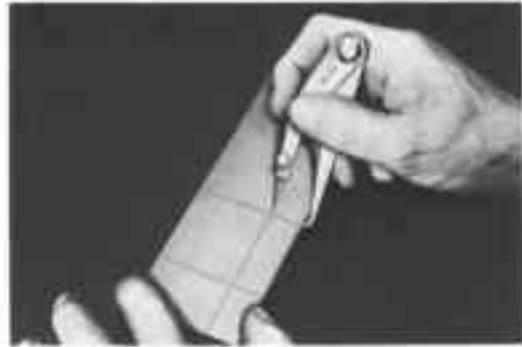
Fig. 3-3. (Left) Using combination square and scribe to lay out plate. (Right) Using hermaphrodite calipers to lay out plate.
