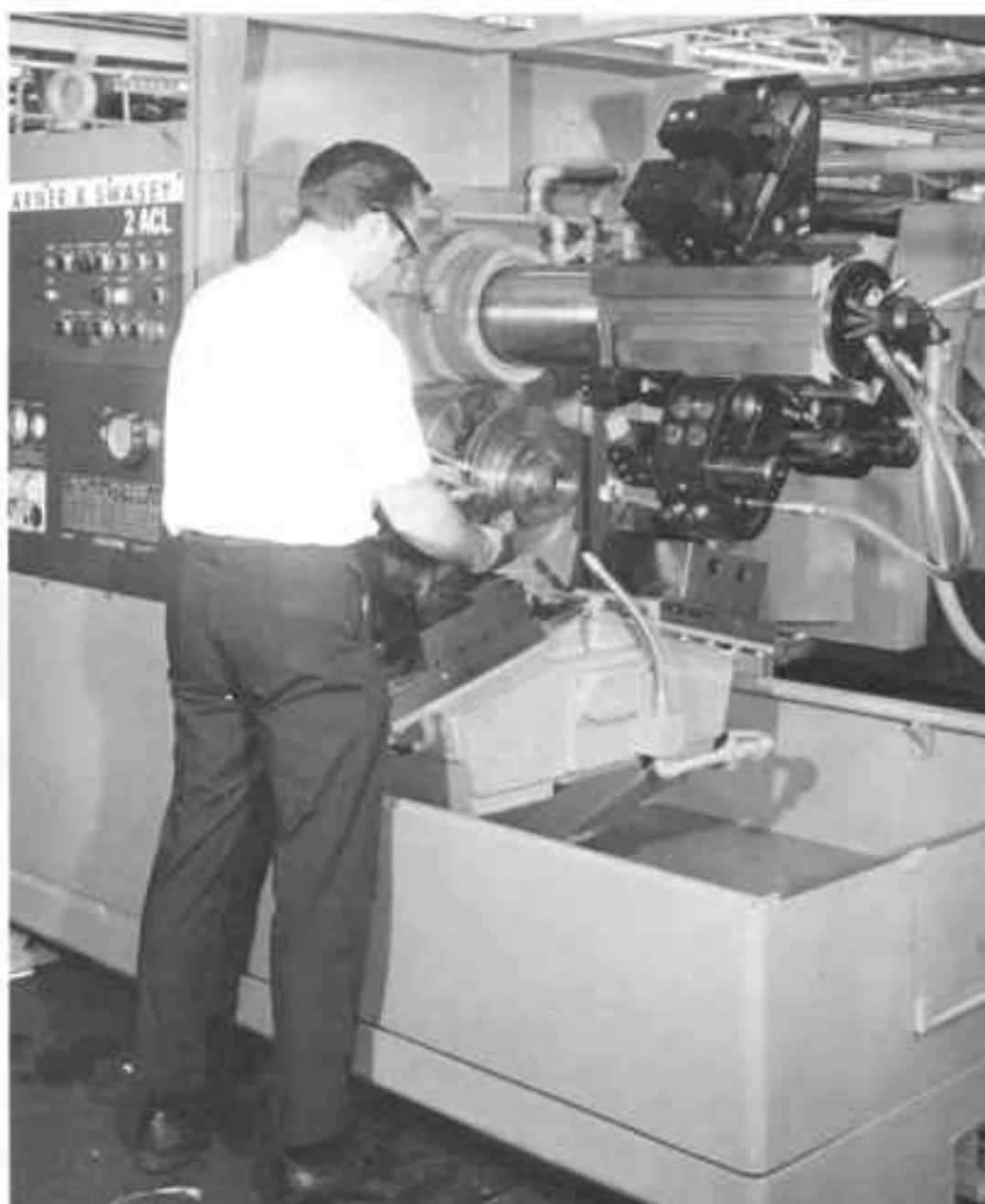
Fig. 4-19. Changing a tool in an automatic chucker.
