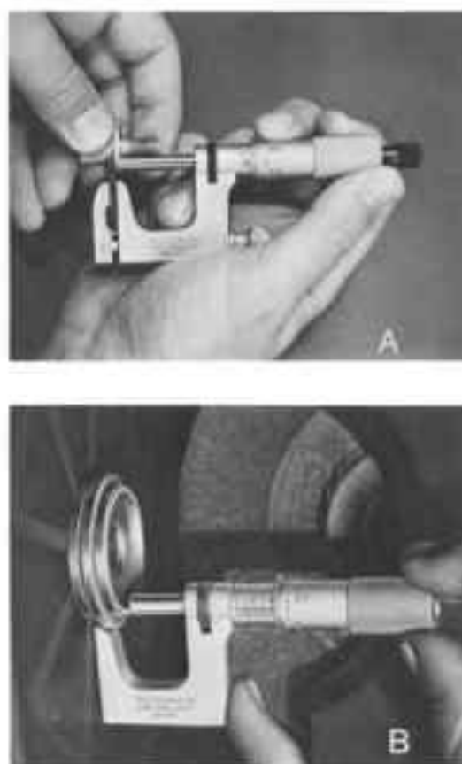
Fig. 2-25. Starrett Mul-T-Anvil micrometer caliper. A. Used as a micrometer caliper. B. Used as a height gage to measure part on surface grinder.
