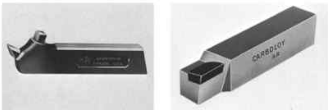
Fig. 7-5: A. (Left) Toolholder for high-speed steel tool bits, B. (Right) A cemented-carbide cutting tool with a brazed-on insert.
