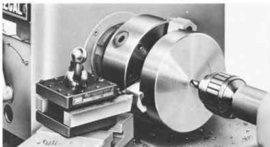
Fig. 9-19. Drilling a small-diameter hole with a drill held in a drill chuck which is mounted in the tailstock spindle.
