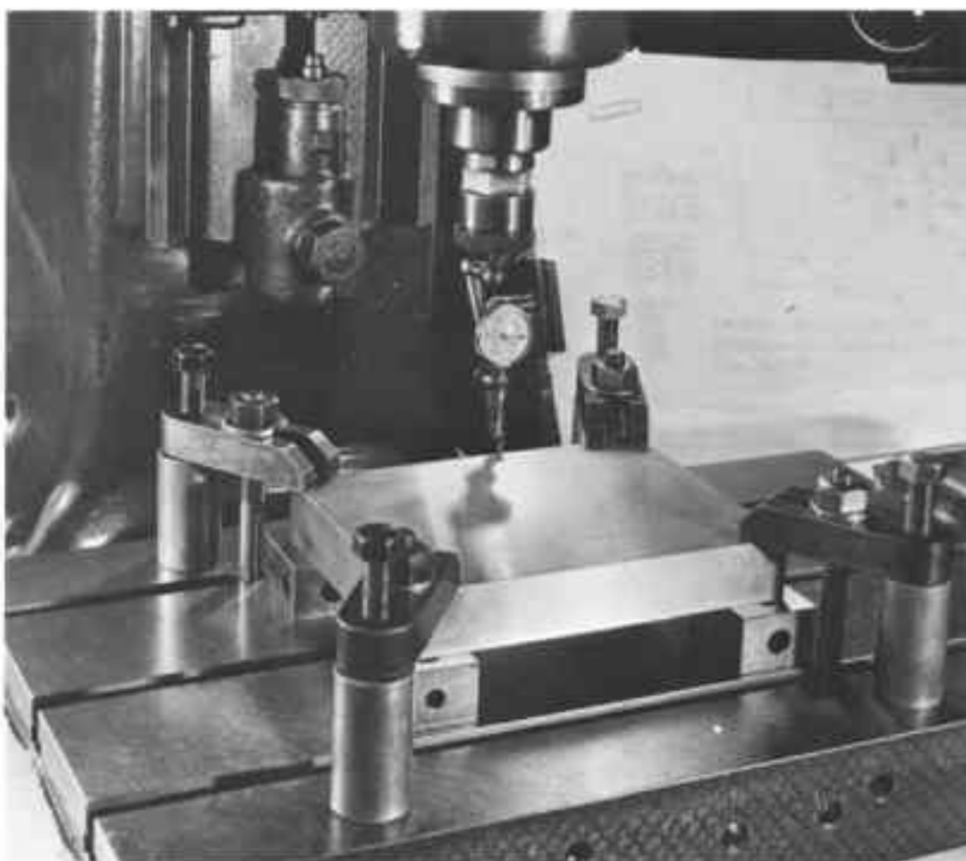
Fig. 15-18. Indicating the edge of a die block to align it with the longitudinal table movement.
