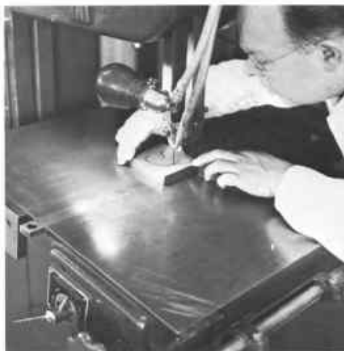
Fig. 16-15. Sawing a blanking punch and die in one operation, with the work table tilted.
