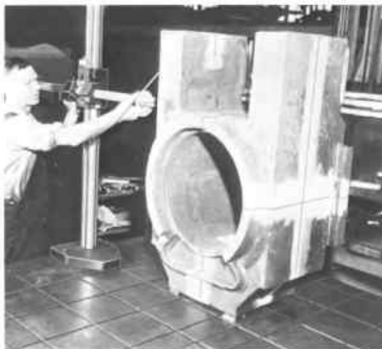
Fig. 3-19. Laying out a large casting with a layout machine.
