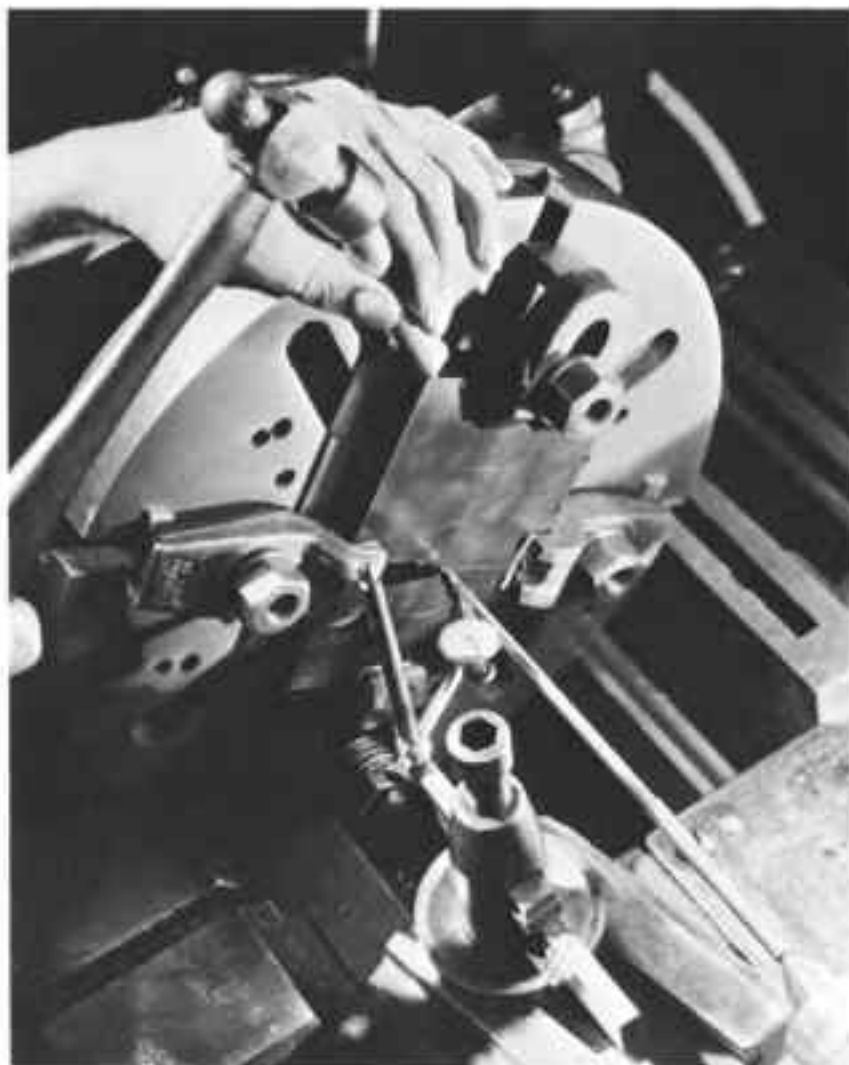
Fig. 15-8. Aligning the work with the axis of rotation of the lathe using a pump center and an indicator.
