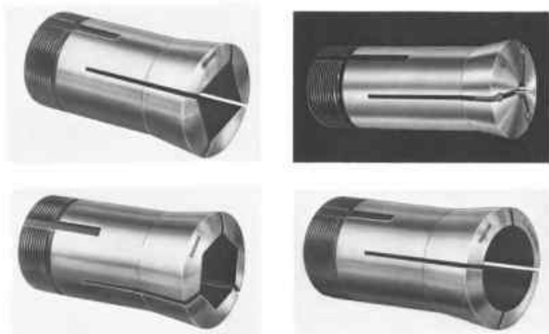
Fig. 9-8. Spring collets for holding different work shapes.
