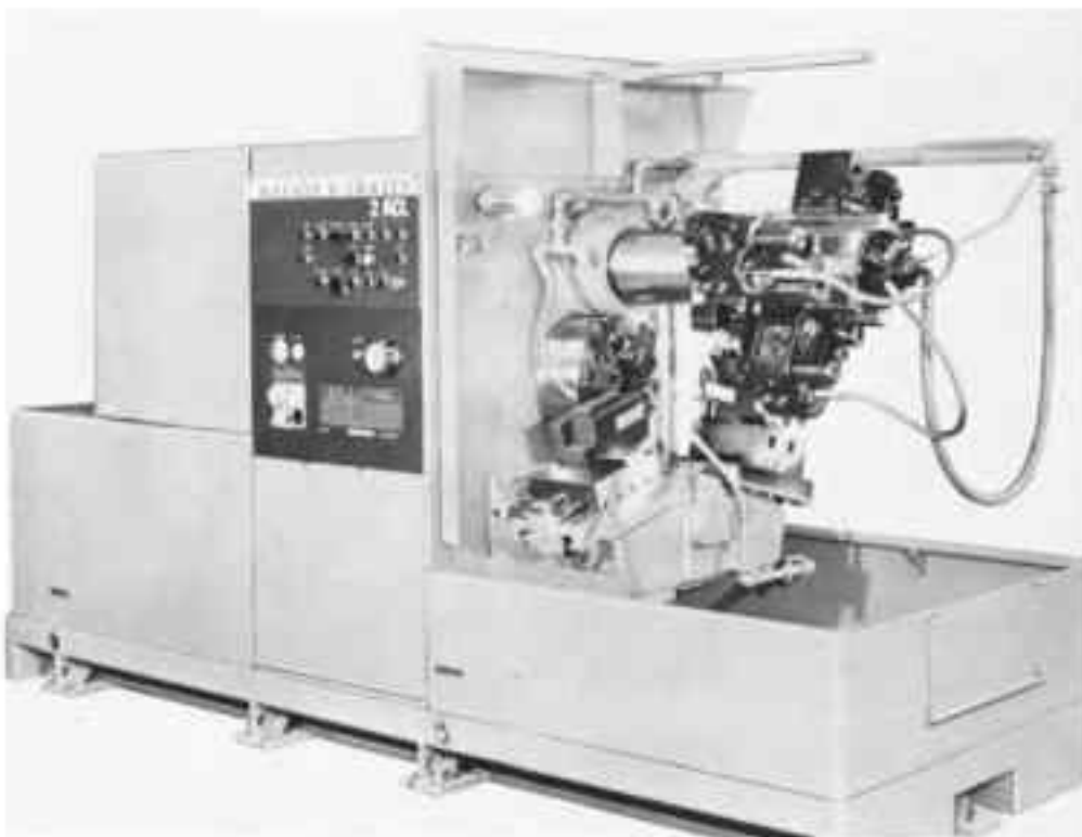
Fig. 14-18. A single-spindle automatic chucking machine.
