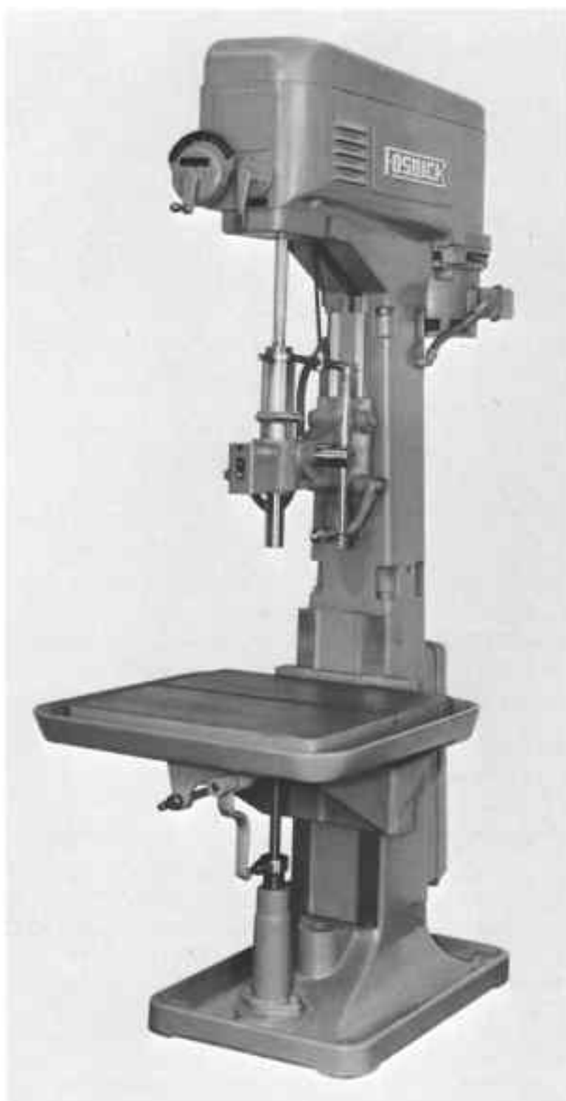
Fig. 4-2. Sensitive upright drilling machine—box column, square-table type.
