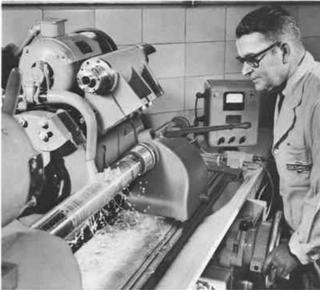
Fig. 1-6. Principle of cylindrical grinding, "traverse" method.
