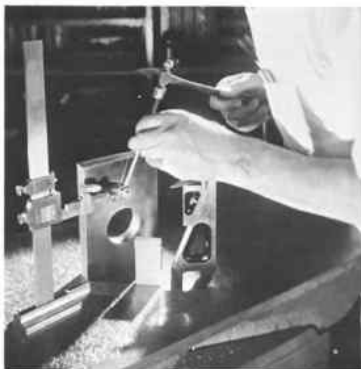
Fig. 15-12. Locating the button on the workpiece. This must be done in two directions from two reference edges.
