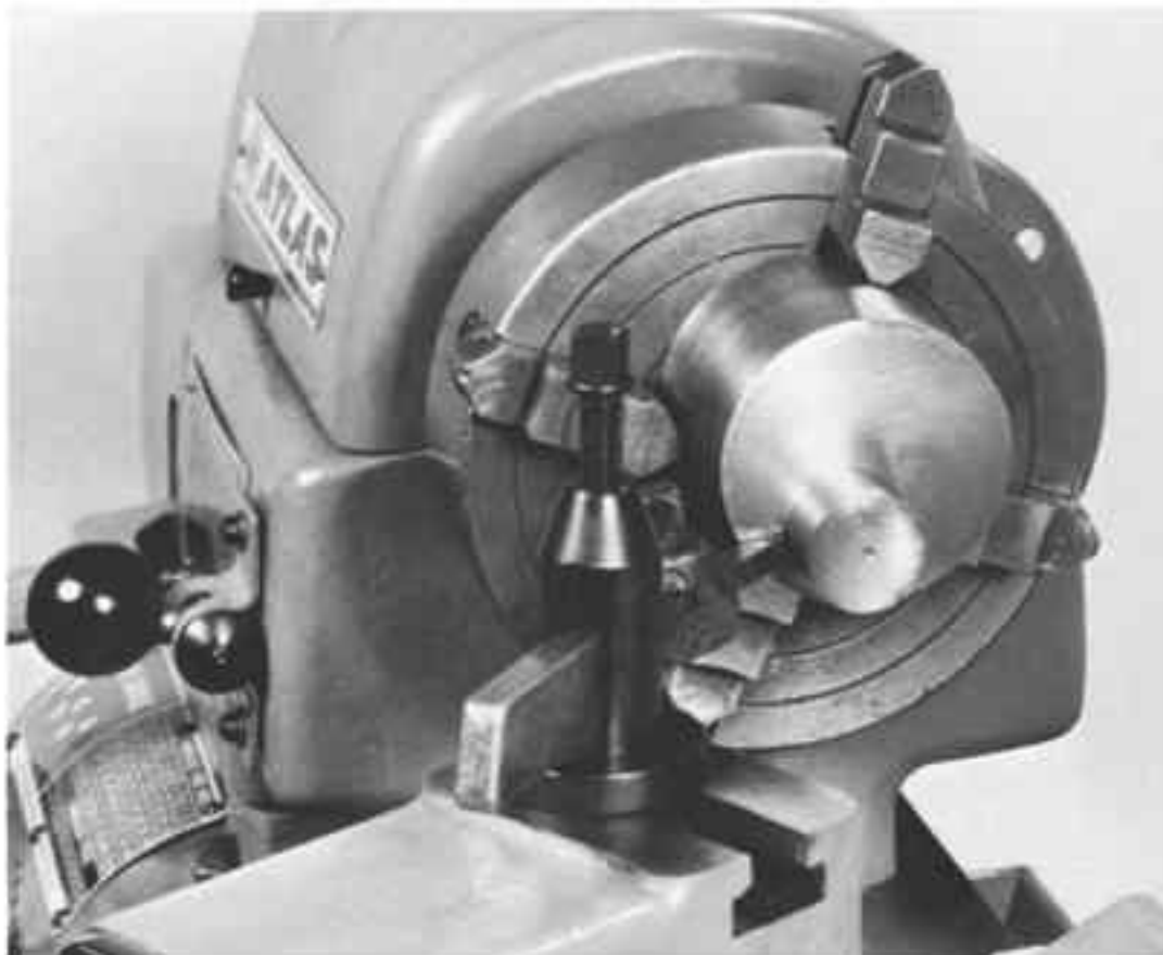
Fig. 9-7. Work held eccentrically in a 4-jaw independent chuck.
