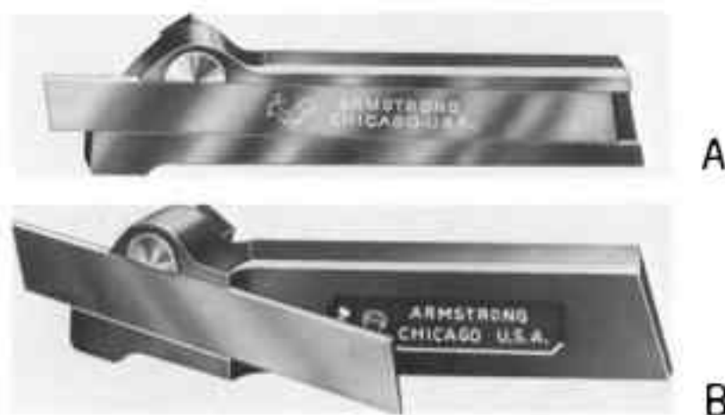
Fig. 9-29. A. Straight-shank cut-off tool. B. Offset-shank cut-off tool.
