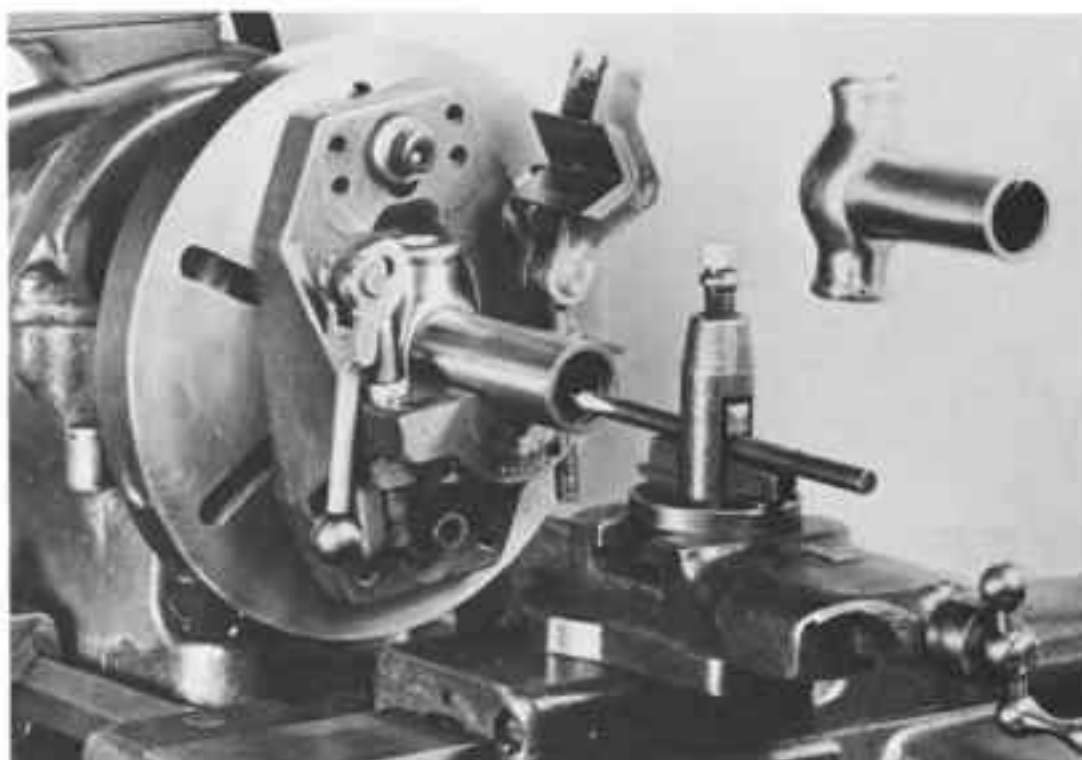
Fig. 11-10. V-block angle plate attached to faceplate and used to hold T-shaped part.
