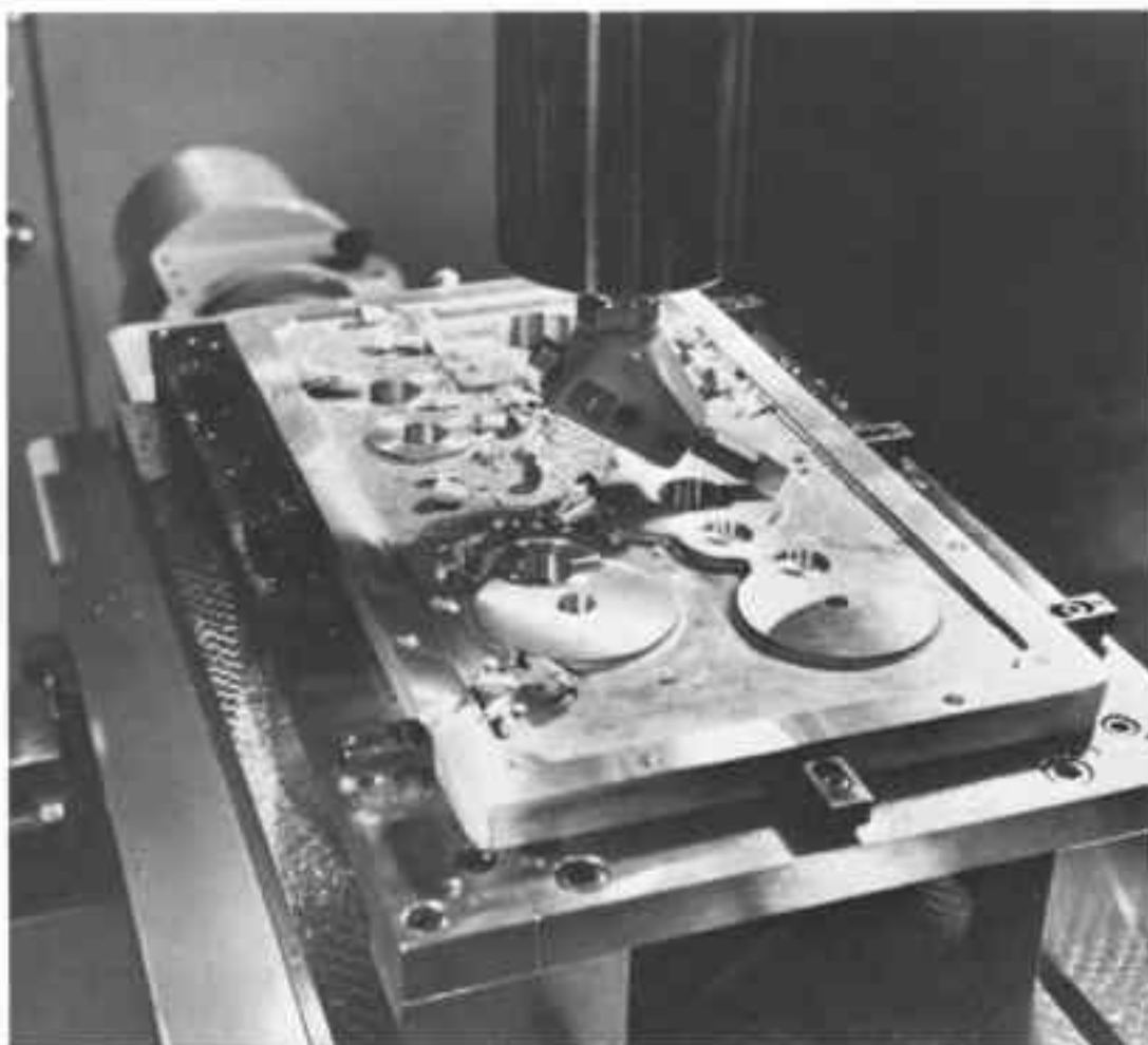
Fig. 15-35. Using a fly cutter to mill a large surface area on a jig-borer.
