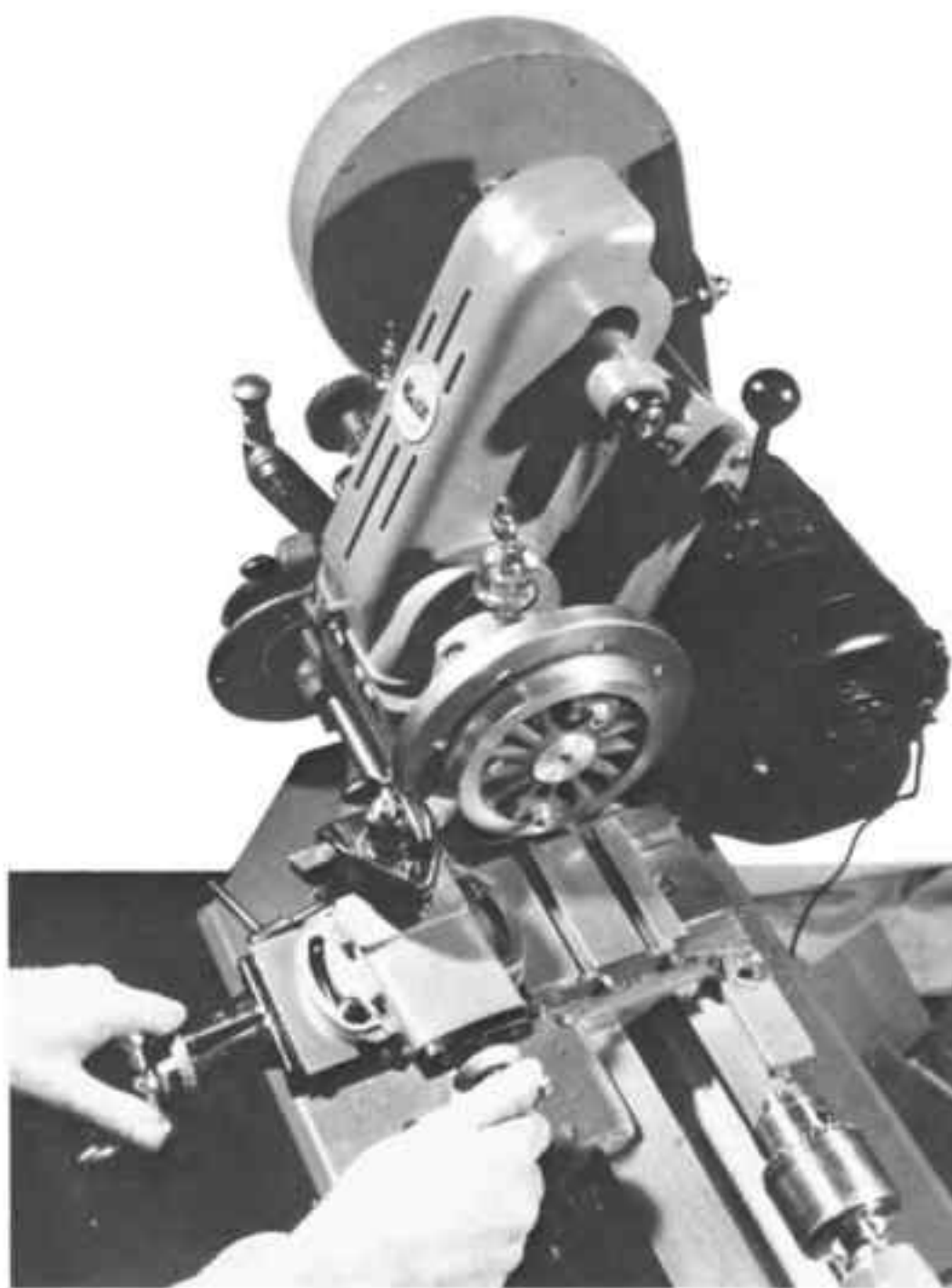
Fig. 11-16: Machining a model steam-locomotive driving-wheel which is mounted on a faceplate.
