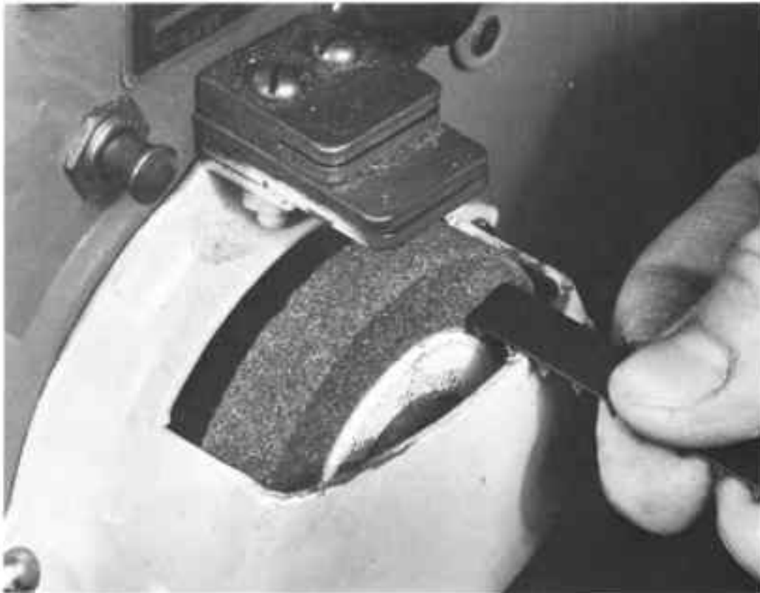
Fig. 16-11. Grinding end of band-saw blade in preparation for welding. Note saw teeth on opposite sides.
