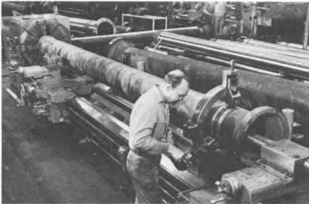
Fig. 6-24. Boring a large workpiece in a lathe with the end held by a steady rest.
