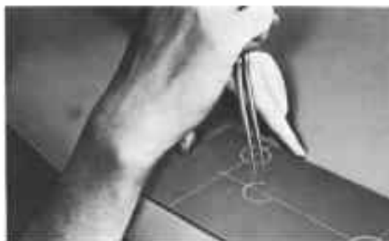
Fig. 3-2. Scribing hole diameters on a hole layout using spring dividers.
