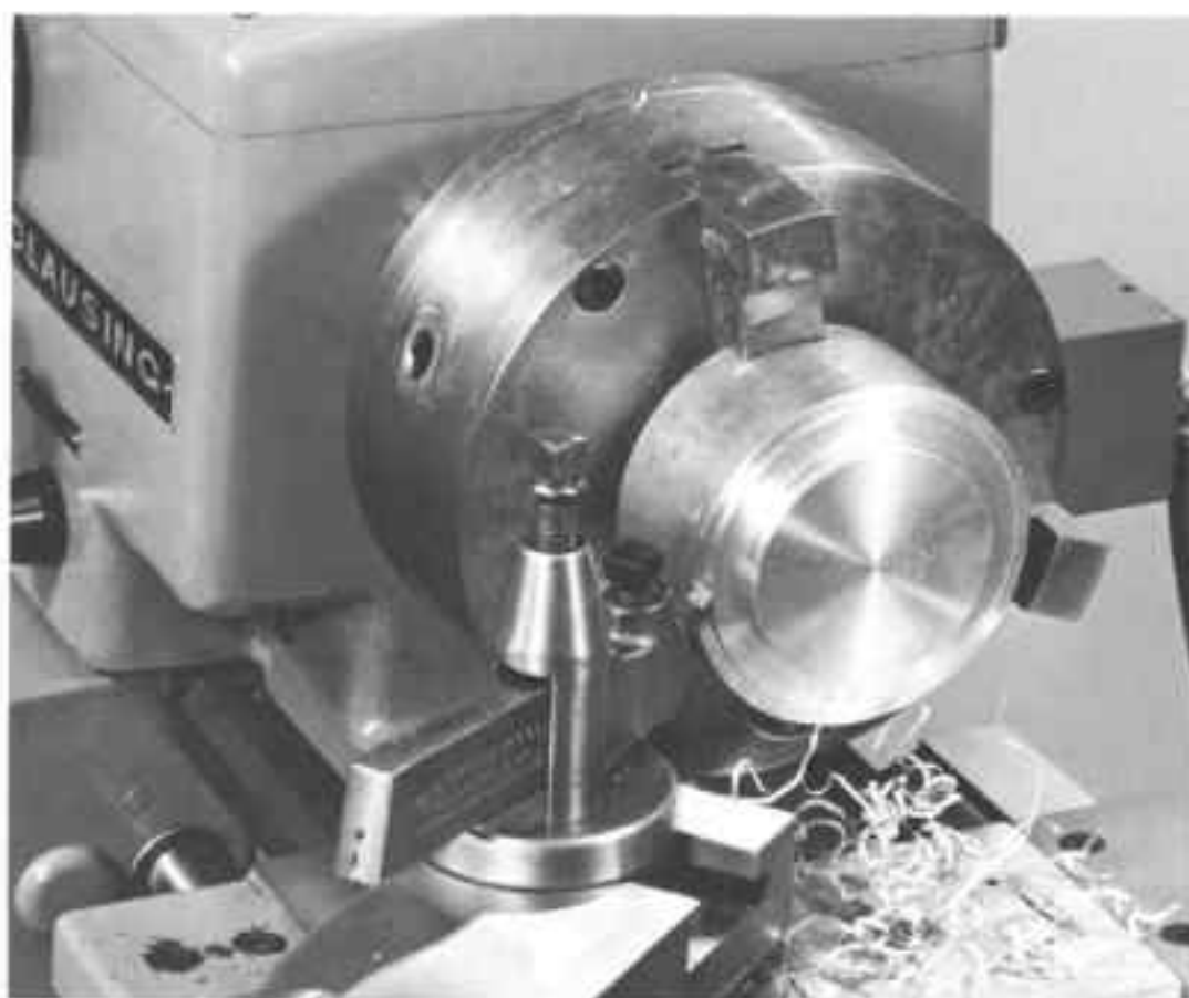
Fig. 9-16. Turning a part that is held in a 3-jaw universal chuck.
