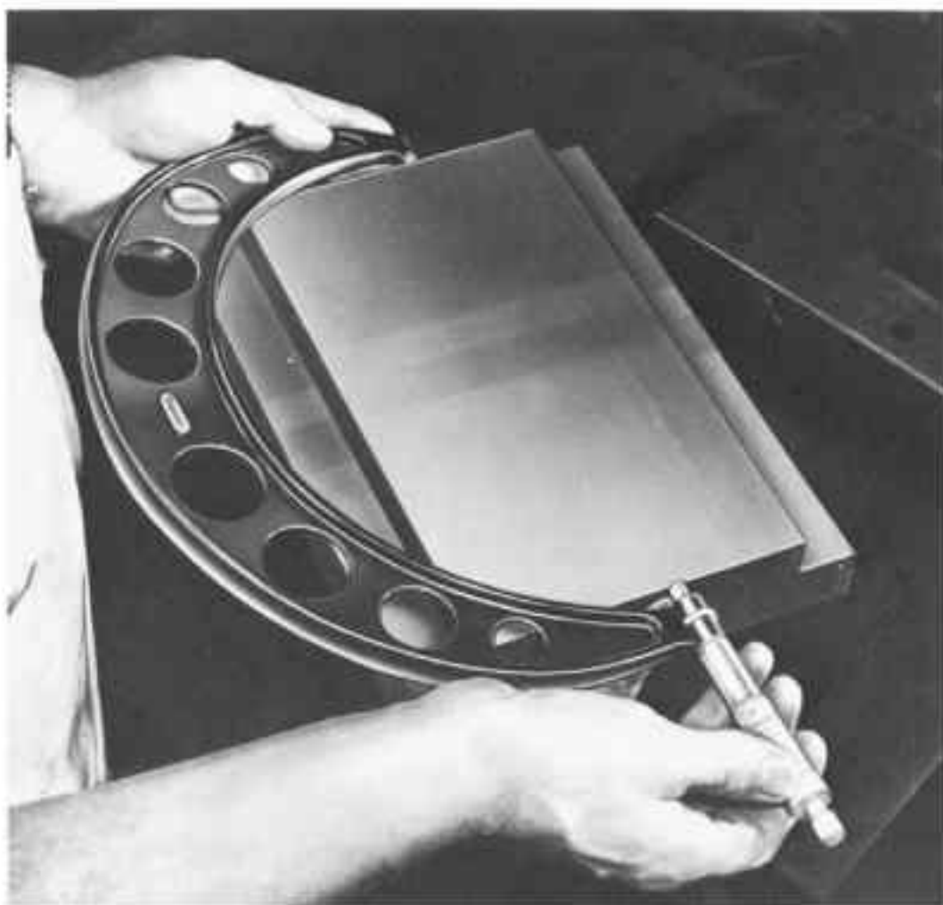
Fig. 2-22. Measuring with large outside-micrometer caliper.
