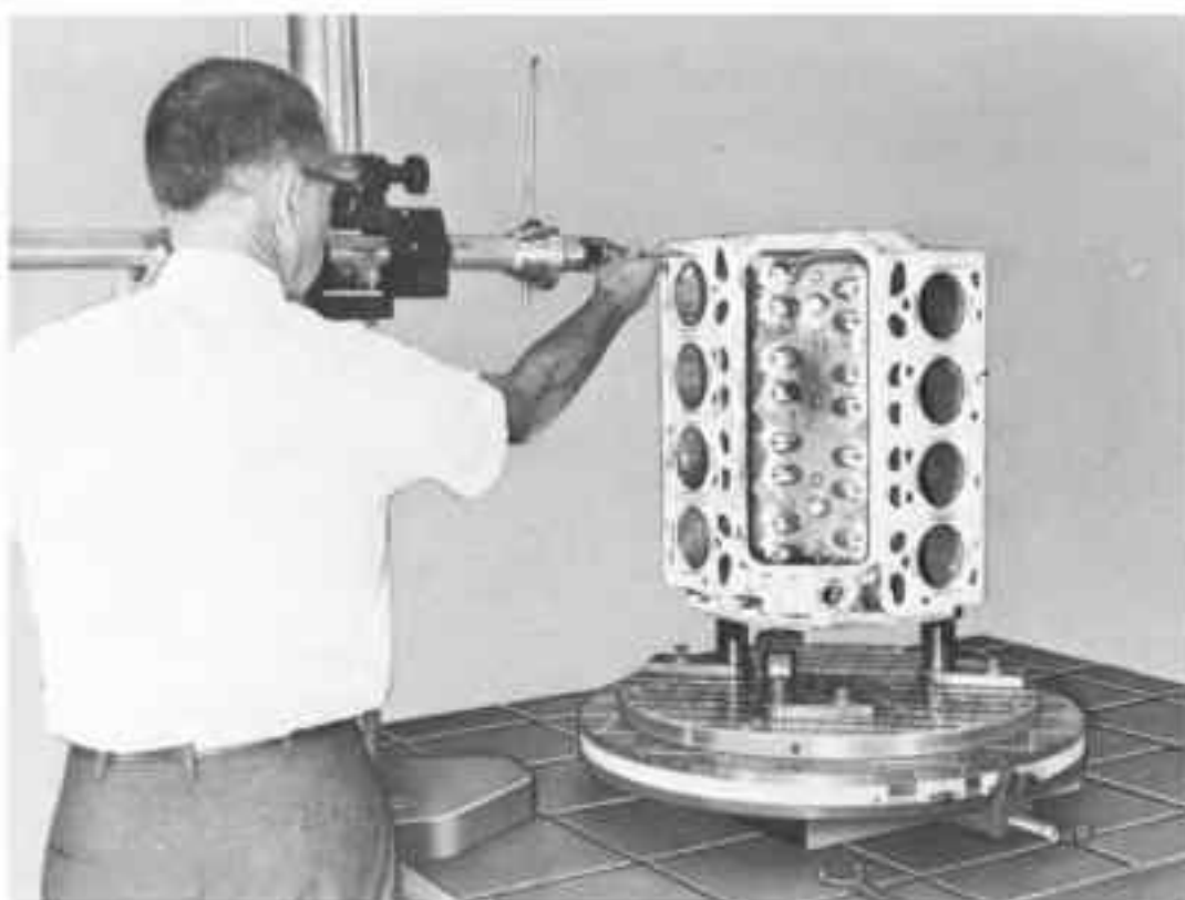
Fig. 3-17. Layout machine used to lay out a cylinder block.
