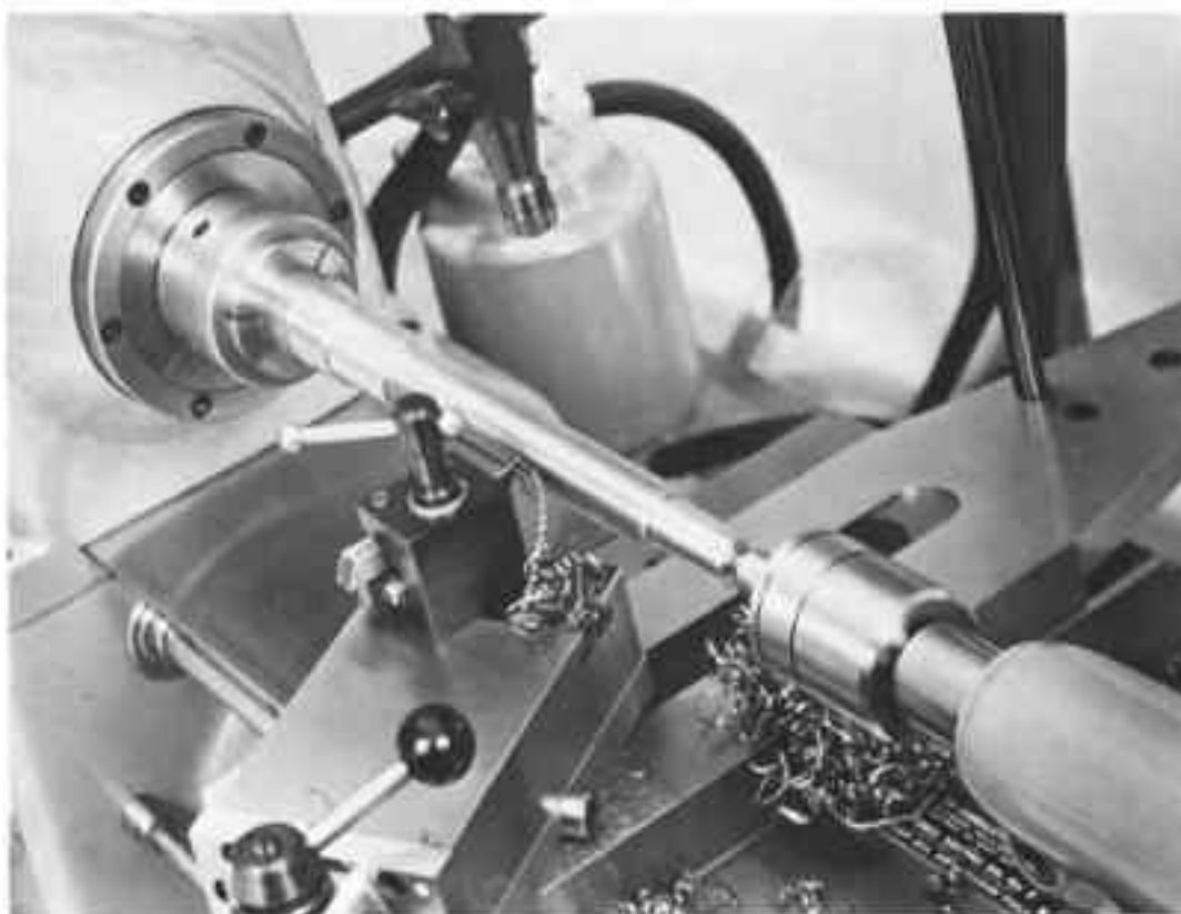
Fig. 13-17. Cutting an American Standard Unified thread on a precision toolmakers' lathe with work held in a collet chuck and on a center.
