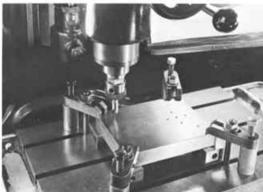
Fig. 15-26. Spot-drilling holes in a die block on a jig borer.
