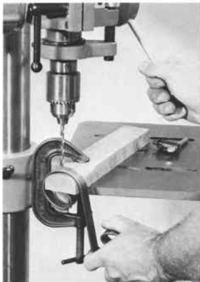
Fig. 5-8. Drilling an ornamental iron part using a wood "fixture," which is clamped to the table.
