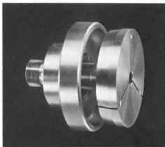
Fig. 9-12. Step chuck, showing closing ring and collet, which is usually called "the chuck."
