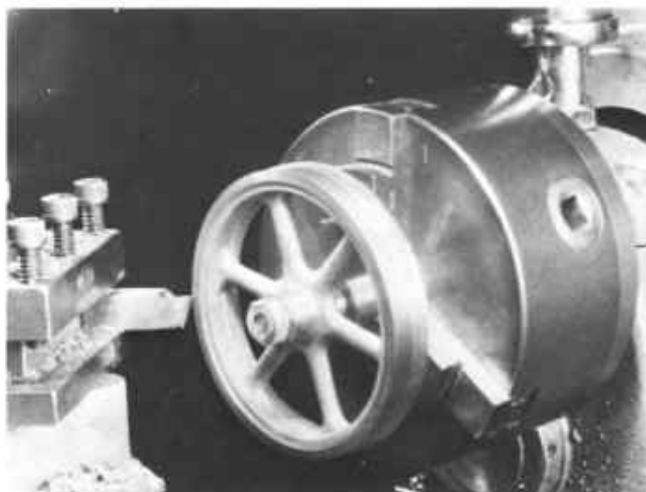
Fig. 9-31. Stub mandrel used to align bore of workpiece with axis of lathe to insure concentricity and perpendicularity of turned surface with bore.
