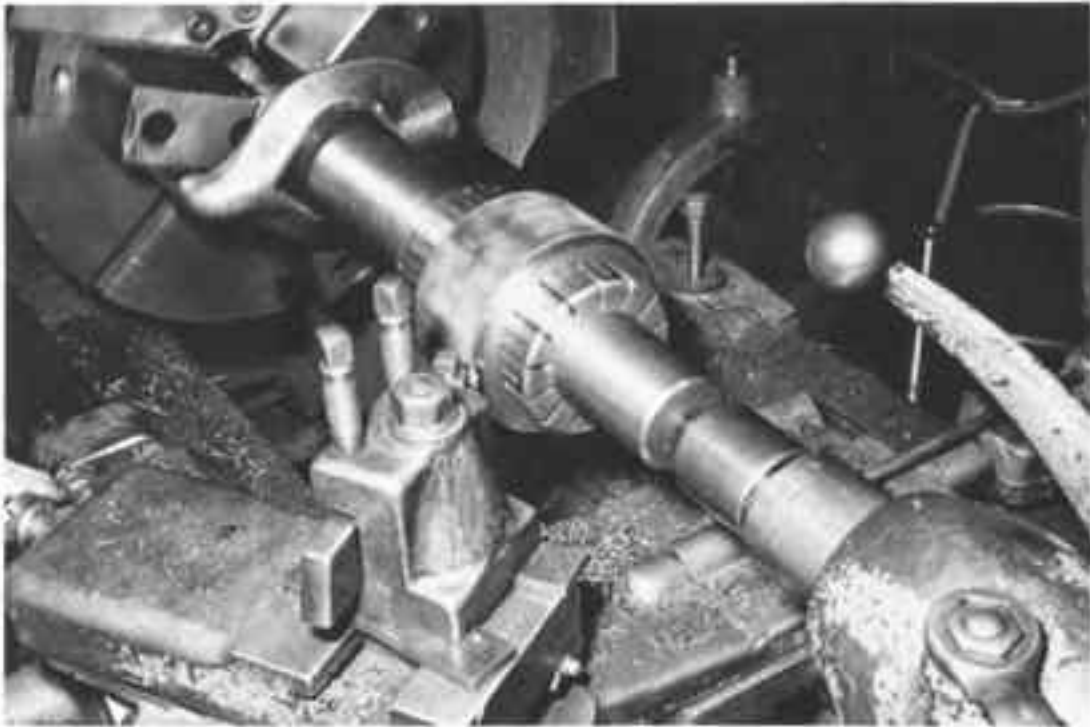
Fig. 8-26. An expanding mandrel used to hold a bushing while turning a short taper using the compound-rest.
