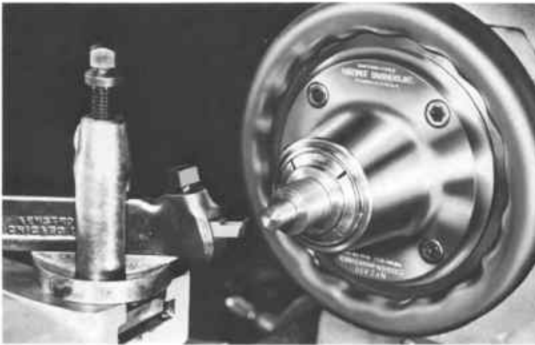
Fig. 9-14. Turning and facing a part held in a spindle nose type collet.
