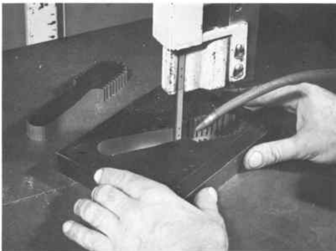
Fig. 16-20. Filing the block of the die using a file band.
