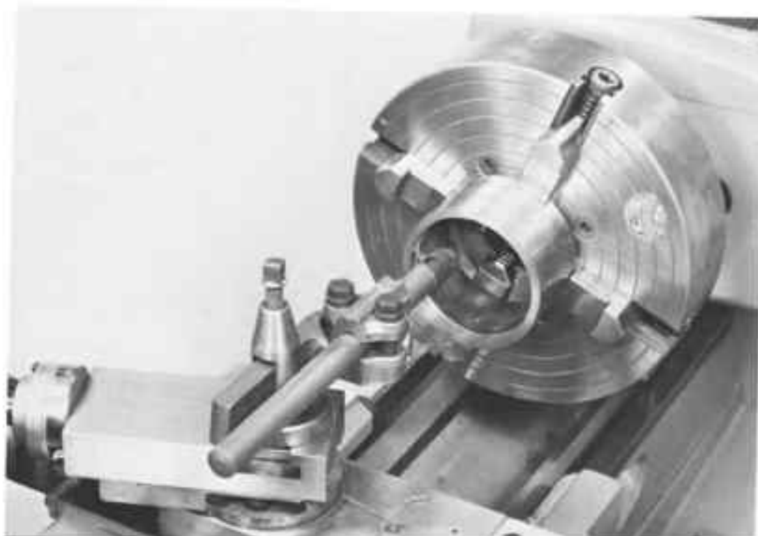
Fig. 9-24. Boring a hole on an engine lathe.
