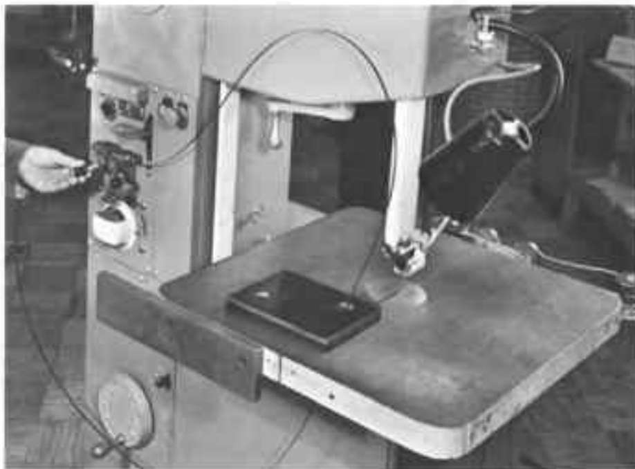
Fig. 16-13. Welding a band-saw blade together in preparation for making an inside cut on the part.
