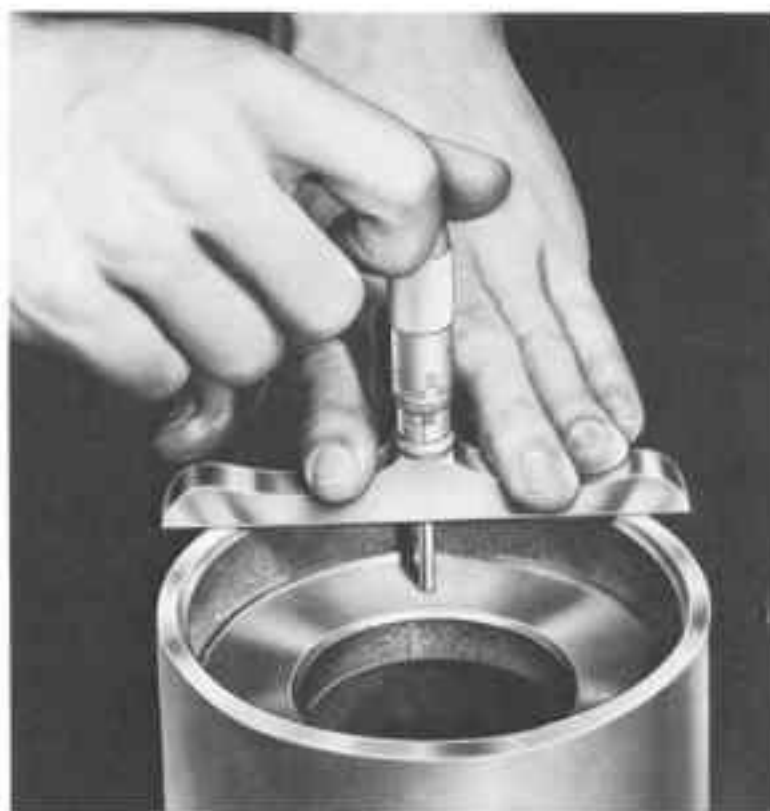
Fig. 2-24. Using depth micrometers to measure shoulder depth.
