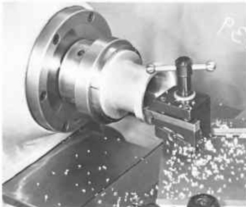
Fig. 9-13. Step chuck holding workpiece to perform turning, facing, boring, and counterboring operations.
