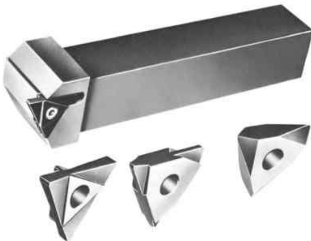
Fig. 7-10. Toolholder and inserts for thread cutting and for cutting shallow grooves. Insert is clamped on side of toolholder.
