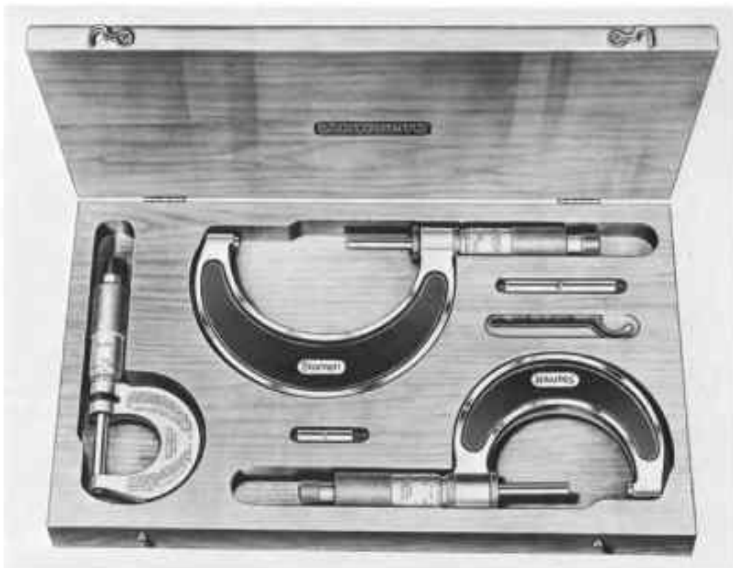
Fig. 2-18. Outside micrometer caliper set including length standards.
