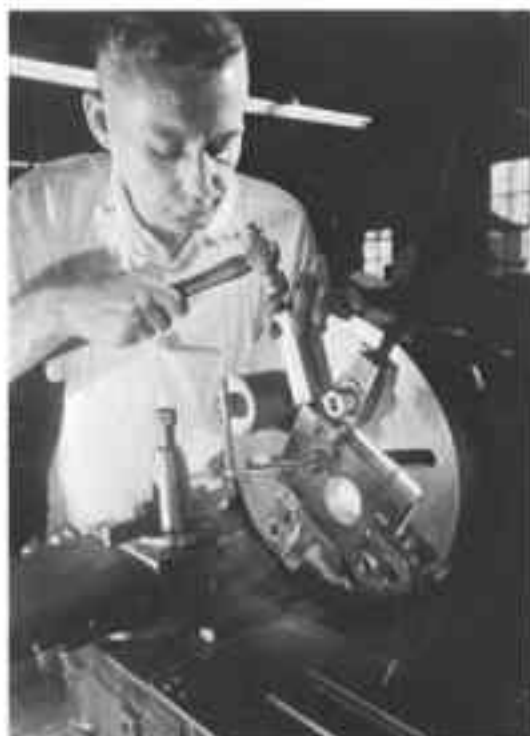
Fig. 15-13. Aligning the workpiece in the lathe with a toolmakers button.
