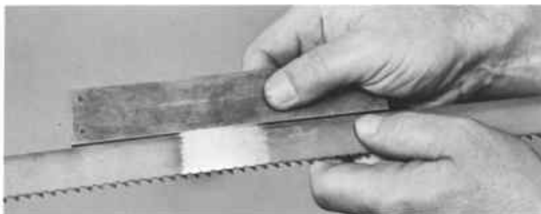
Fig. 16-14. Example of a perfect hand-saw-blade weld.
