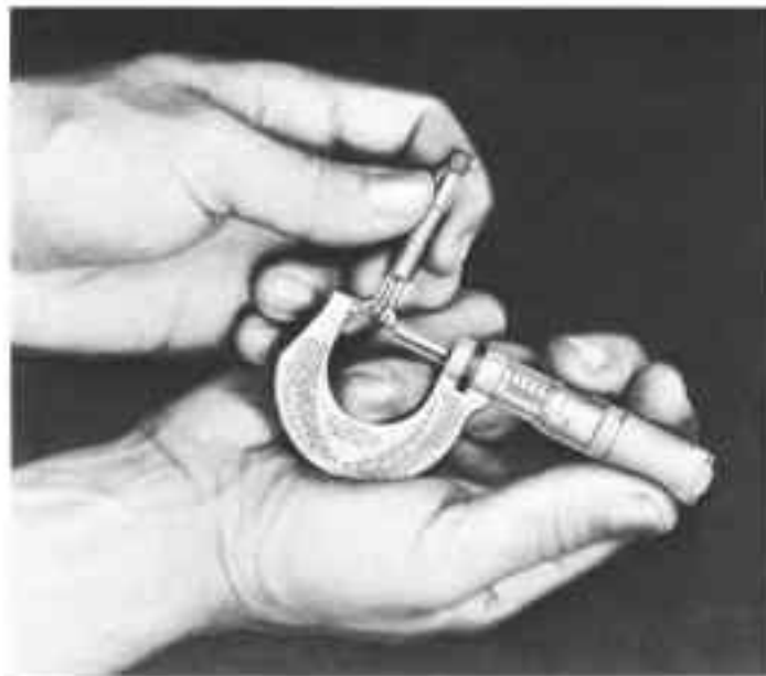
Fig. 2-7. Small hole gage-setting measured by outside-micrometer caliper.
