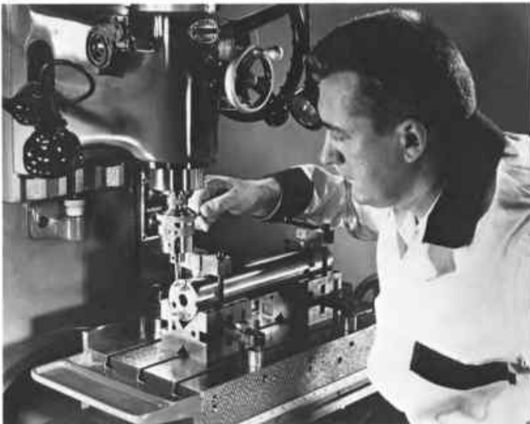
Fig. 15-32. Cylindrical workpiece set up on precision V-blocks for jig-boring.
