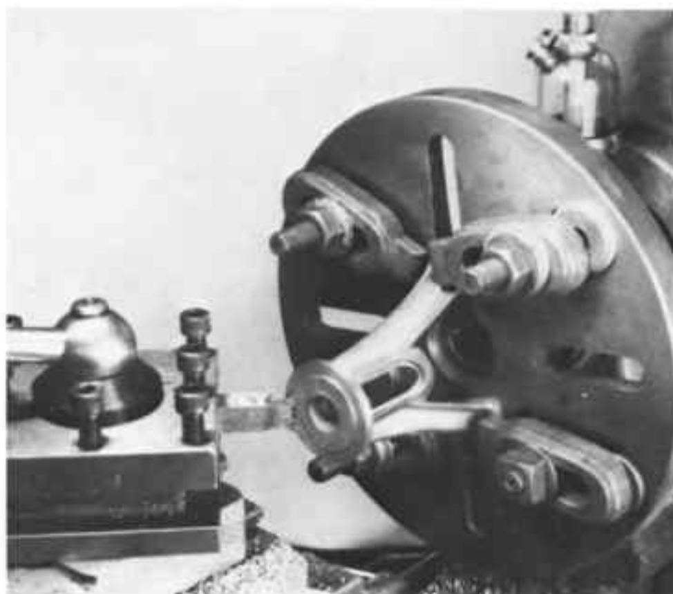
Fig. 11-17. Facing a model steam-engine trunk-column casting.
