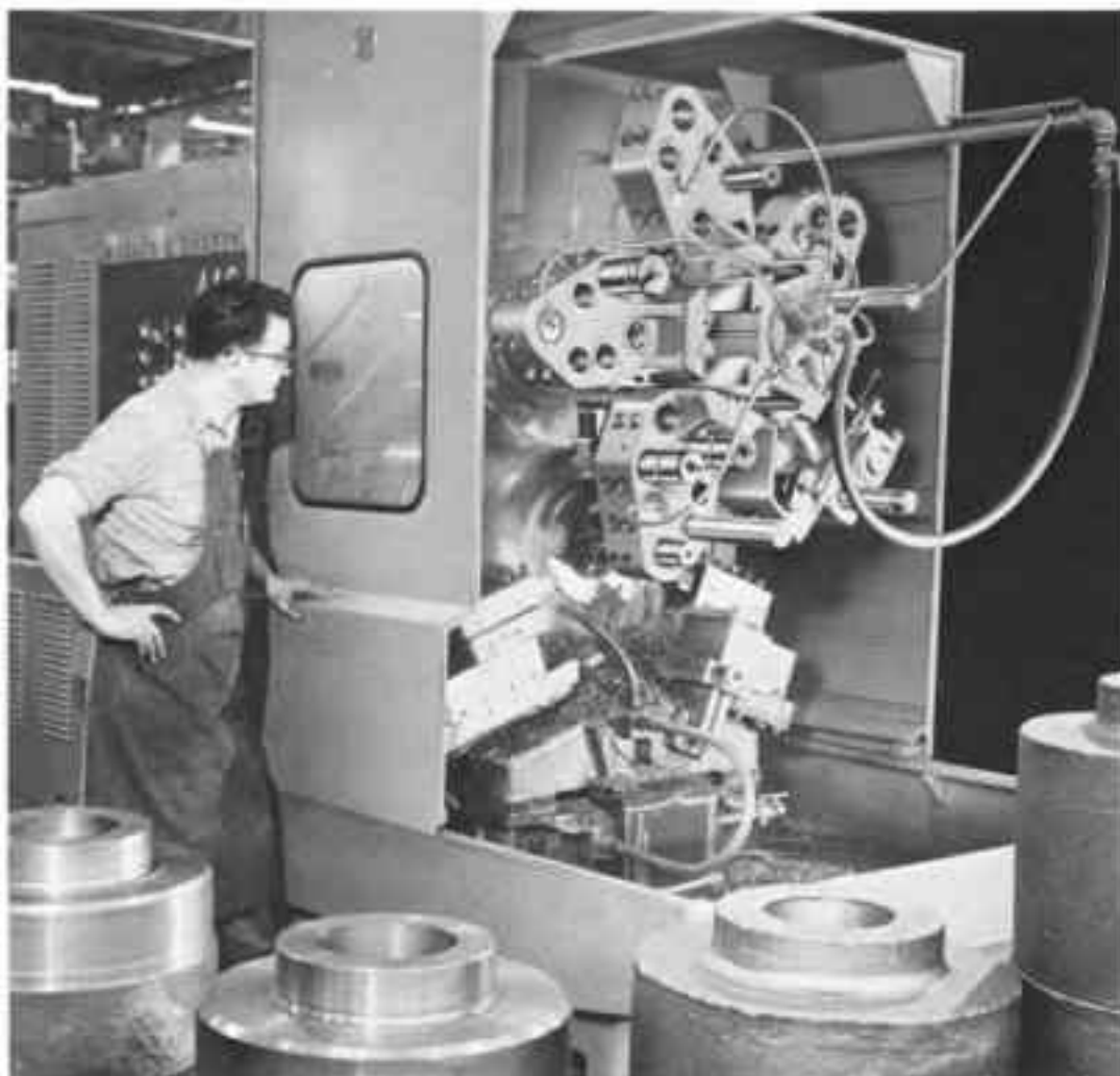
Fig. 14-20. Machining heavy castings in an automatic chucker.
