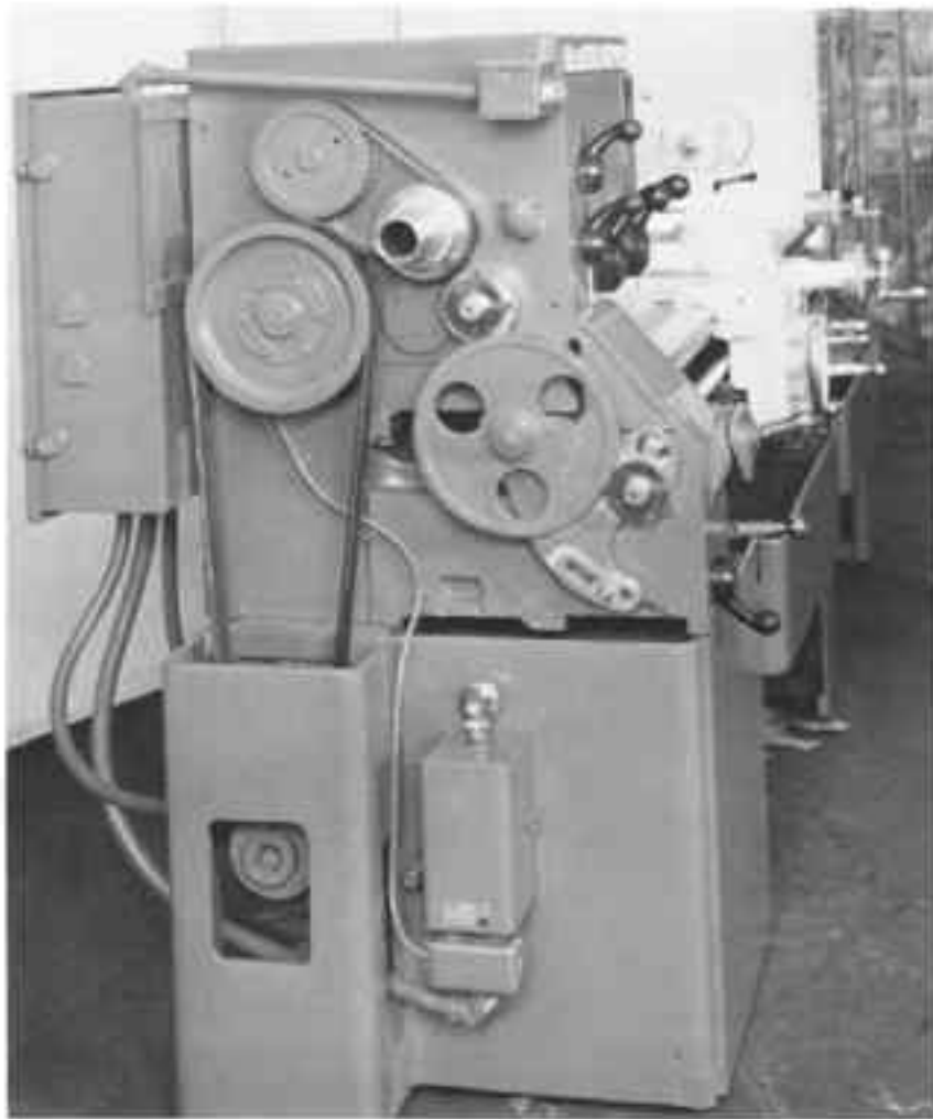
Fig. 6-14. Front end of engine lathe showing gear train from headstock spindle to quick-change gearbox. The pick-off gears in the train can be quickly removed and replaced by other gears.
