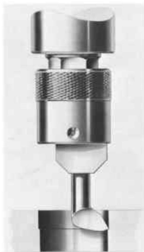
Fig. 15-3. Single-point boring—the most precise hole-locating method. The surface is generated by rotation about the hole axis. Either the workpiece or tool may rotate.
