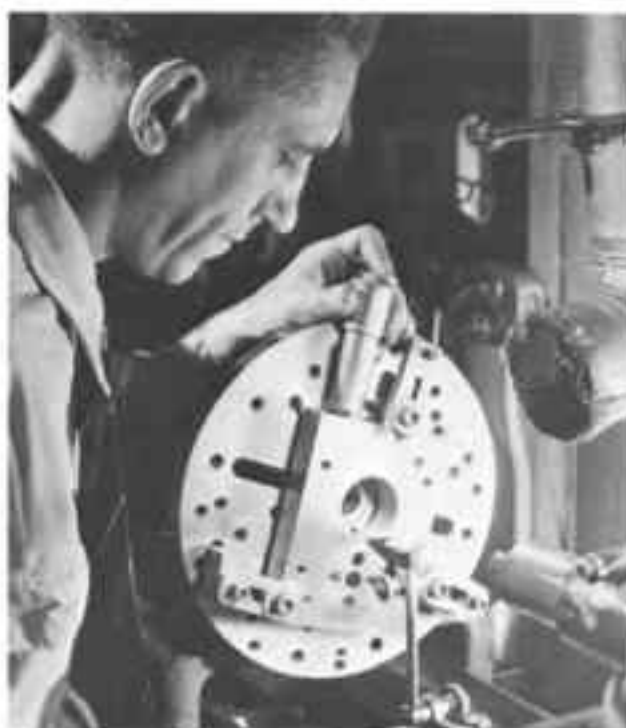
Fig. 15-38. Locating a blanking die on a faceplate by indicating the hole.
