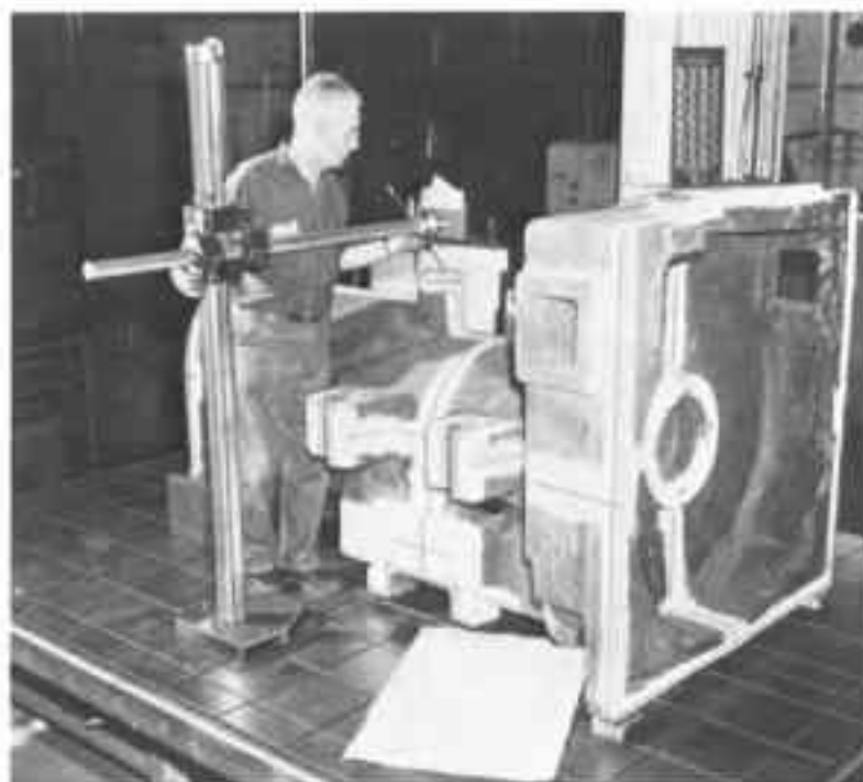
Fig. 3-18. Laying out a large casting with a layout machine.
