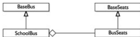
Figure 9-11: The difference between inheritance and aggregation/composition
