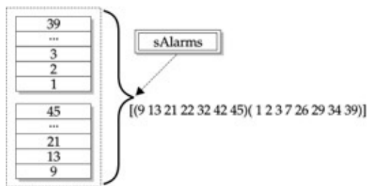
Figure 12–10: The array after it has been partitioned
