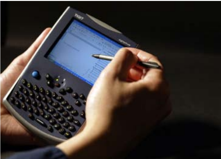
Figure 3: The Tiquit Eighty Three Computer. This device provides a keyboard, a joystick and a stylus for user interaction.
