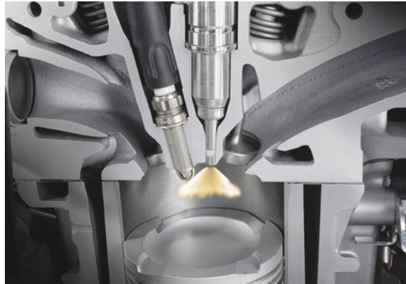
Fig. 4.35 Example of a centrally arranged injector with homogeneous direct injection, Mährle et al. (2007)
