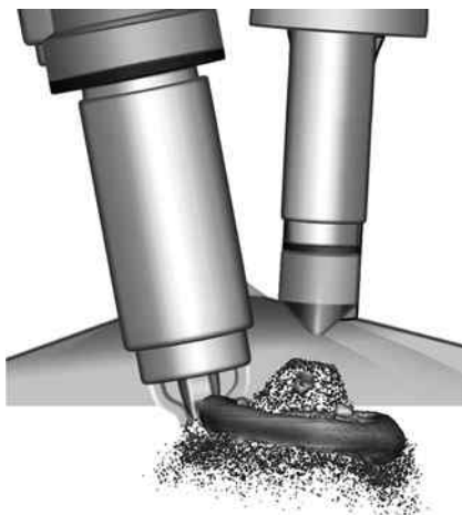
Fig. 4.38 Increasing the HC mass flow at operating point 2,000 rpm, w_e = 0.2 kJ/l in the wall-guided process compared to stoichiometrically operated engines, Göschel (2006)
