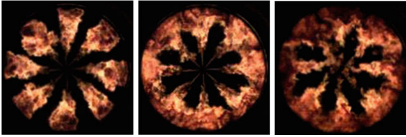
Fig. 3.38 Flame distribution seen through the piston of an optical research engine, Lindstrom private communication
