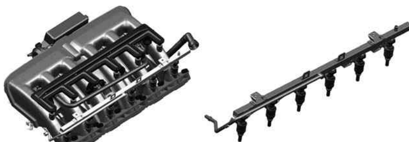
Fig. 4.33 Example of the arrangement of the fuel injection line of a manifold injection system on the intake runners, Albrecht et al. (2000)
