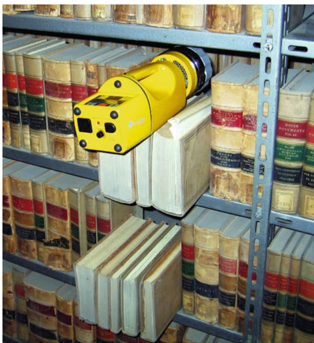
Fig. 9.1 Volumetric sampling of air using a Surface Air System (SAS) instrument in the storage area of a public library. Within the sampler a Petri contact plate coated with nutrient agar is exposed to a flow of air for a pre-defined sampling period
