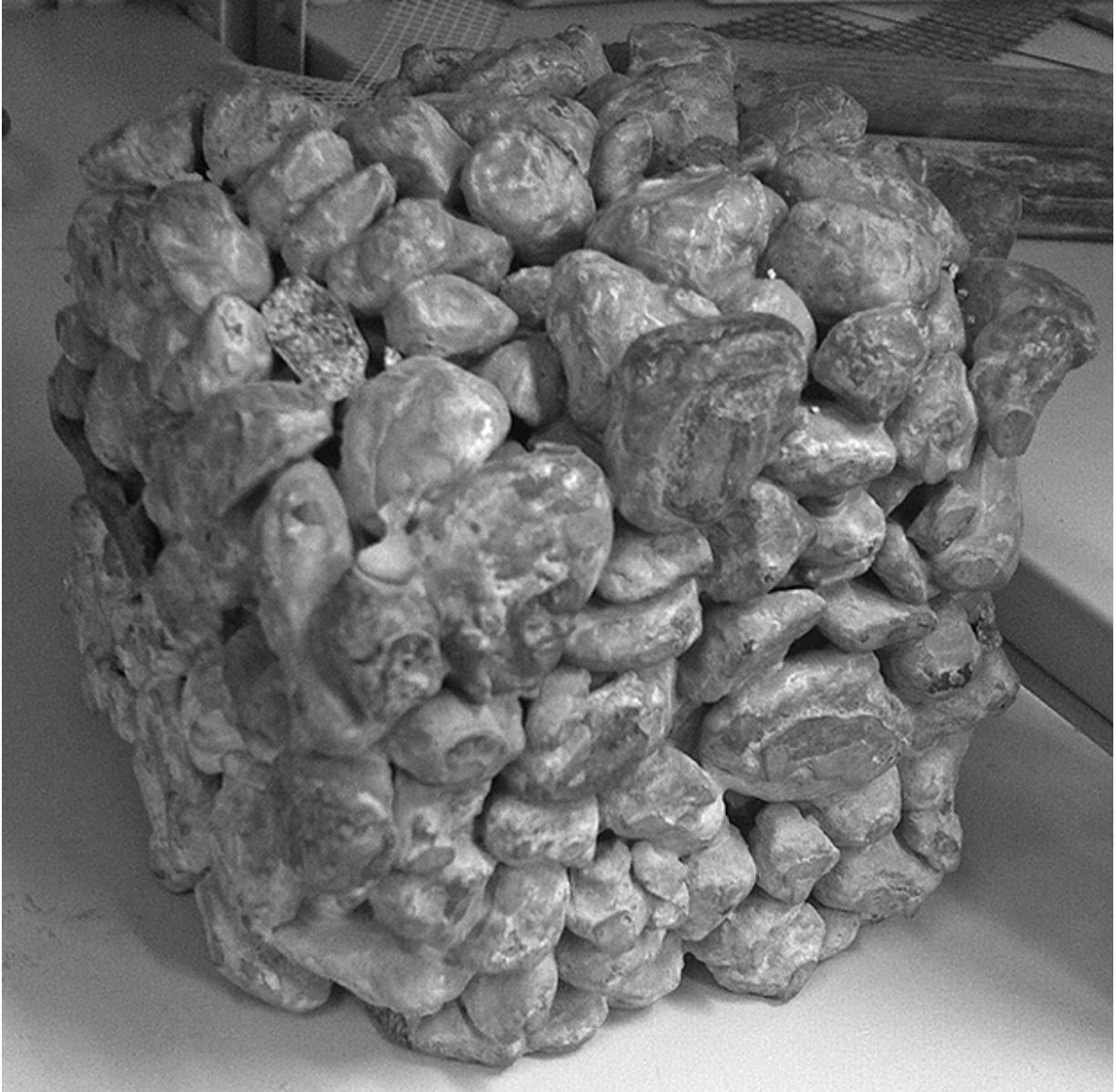
Figure 9.7 A sample of pervious concrete.
