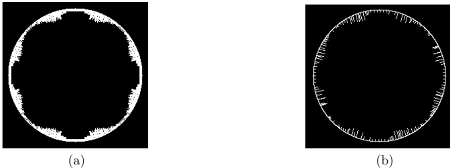
FIGURE 6.13: Normal computation at the contour points for the image circle for B=\{112\} (a) dense normal map, (b) sparse normal map.
