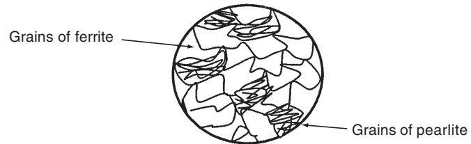
Figure 4.10 Microstructure of mild steel
