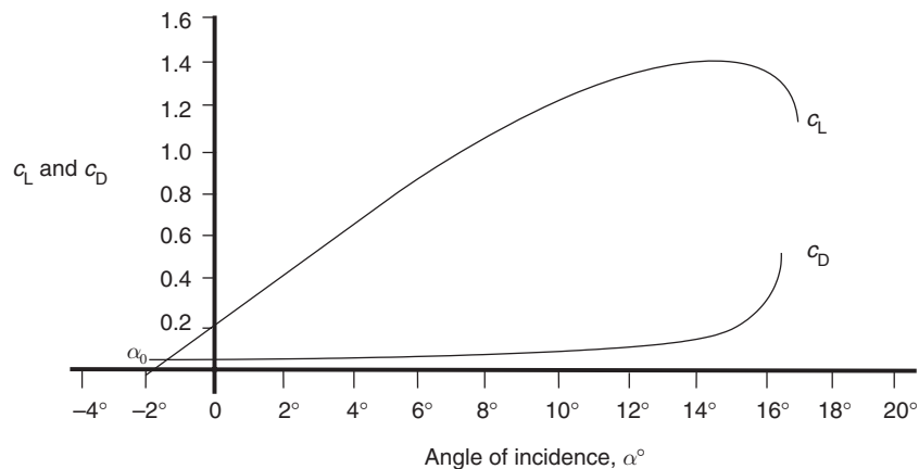
Figure 5.49 Variation of lift and drag coefficients
