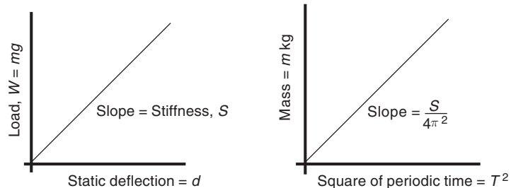
Figure 2.47 Characteristic graphs for mass-spring system
