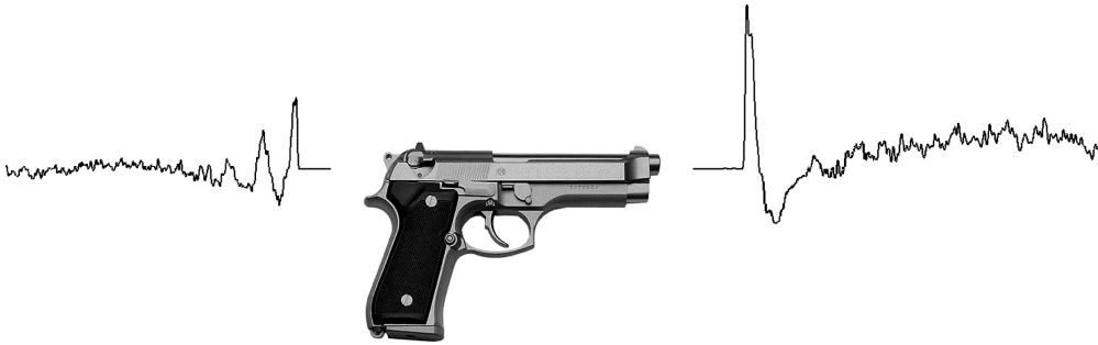
FIGURE 14.6 Directional attributes of muzzle blast wave form.
