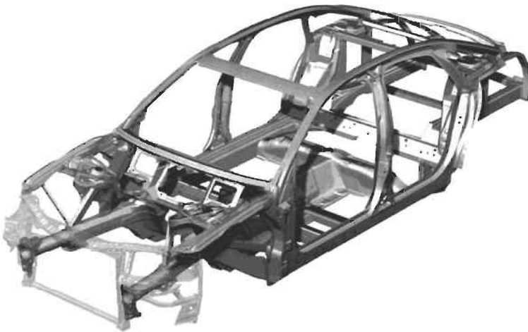
Figure 8.7 The aluminum space frame of the Audi A8.
