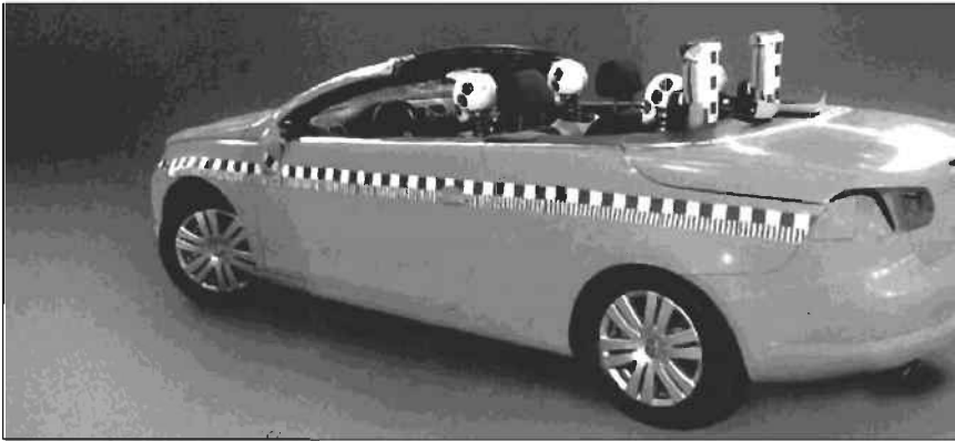
Figure 9.20 Automated rollover protection in a convertible. (Source: Ref: 9-9.)
