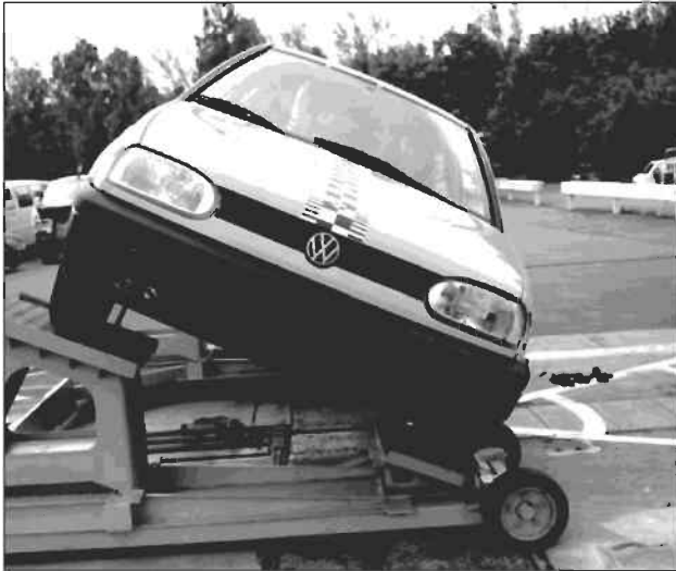
Figure 9.18 Test configuration for the dynamic rollover test in accordance with FMVSS 208.
