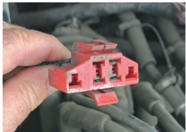
This ABS diagnostic link connector was used on Ford Motor Company vehicles from the early 1980s until 1995. This Ford connector is identical to the Ford OBD-I engine management connector, except for color. On Ford vehicles, the OBD-I connector is black or gray, and located “somewhere” under the hood, at least according to most component locator manuals. Courtesy Elwood’s Auto Exchange
