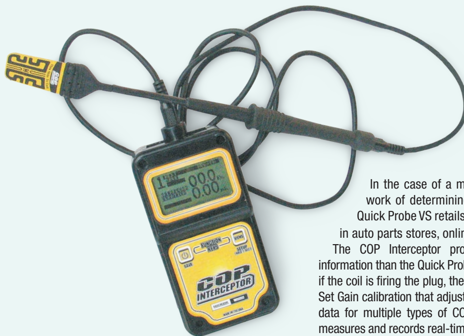
The Weakon COP Interceptor measures, displays, and saves each coil-on-plug's secondary ignition data in real time for detailed ignition analysis. Trend data can be displayed for visual verification of an intermittent misfire that may not trigger a DTC. Courtesy Hickok Inc.
