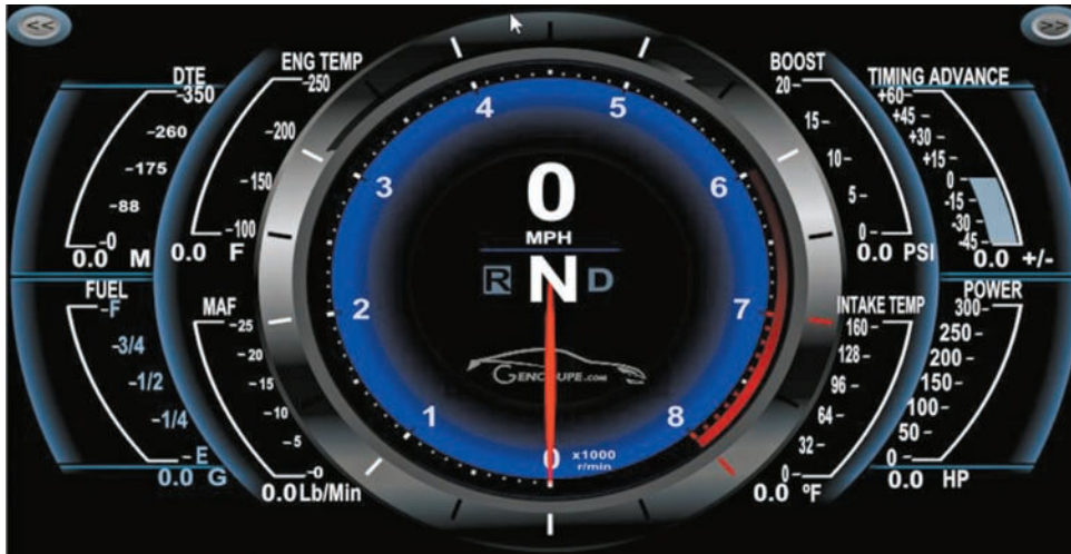
Another DashCommand dashboard. This one shows calculated horsepower in the lower right corner.
