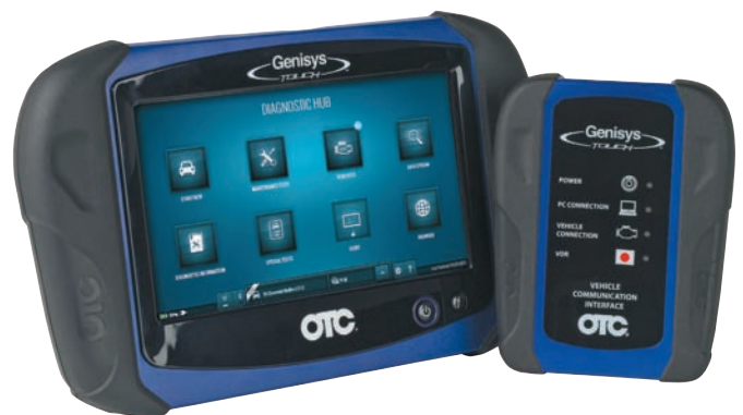
The Genisys Touch is a 10-inch, ruggedized tablet with Bluetooth capabilities. The smaller unit next to the Touch is a vehicle communications interface (VCI) that allows the Touch to connect to a vehicle remotely. Genisys Touch software automatically detects and alerts the technician of on-tool or Web-based repair information. Courtesy SPX/OTC Corporation
