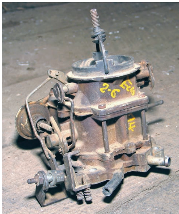
This single-barreled, cast iron carburetor would best be used today as a paperweight, or possibly as a replacement part in a classic car or truck awaiting restoration. Vintage auto parts suppliers still sell rebuild kits for this old hardware. Courtesy Elwood's Auto Exchange
