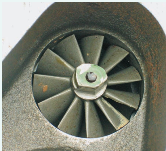
The T3's exhaust turbine wheel is mounted in the exhaust housing of the turbocharger. The irregular shaped metal on the end of the turbine wheel is used to balance the shaft and turbine wheel. Material has been removed to achieve the correct balance.
