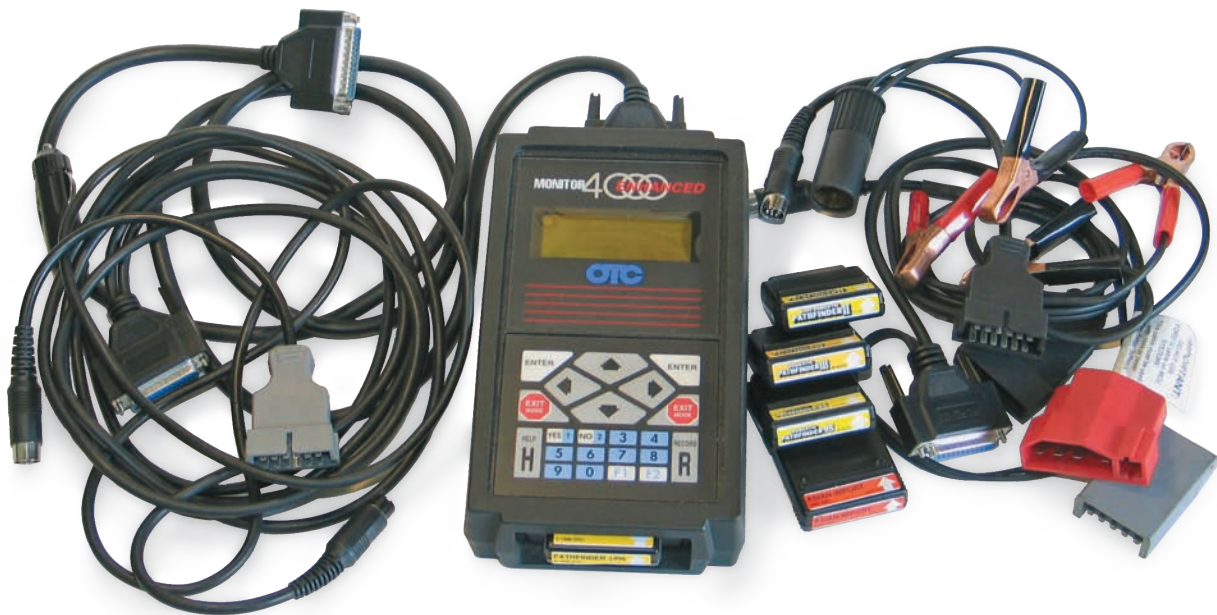
Because manufacturers were not required to standardize OBD-I diagnostic systems, the Monitor 4000E from OTC Tools needed lots of cables and adapters in order to connect to vehicles from General Motors, Ford, Chrysler, and Toyota. The small square boxes to the right of the scan tool are software cartridges for different years and makes of vehicles. This scanner dates from early 1990. At the time, it was much too expensive for home technicians. Courtesy OTC Tools
