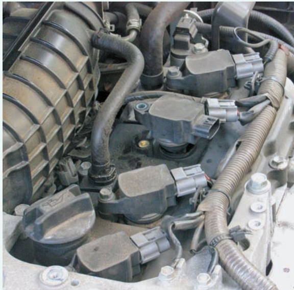
This Nissan 2.4L four-cylinder engine uses coil-over-plug ignition. The four coils can be seen mounted at the top of the valve cover. The coil in cylinder number 3 is about to be removed as the mounting bolt has been taken out and the coil wire harness to the PCM has been unplugged.
