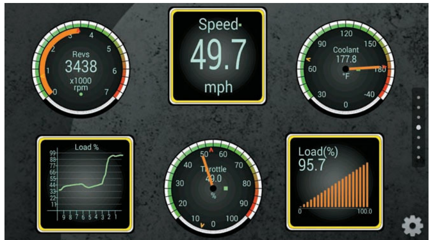
Just one of the numerous dashboard gauge setups that Torque offers. From the top left are: engine rpm, speed in mph, coolant temperature, engine load in a graph format, throttle position in percentage, and engine load in a bar graph format.
