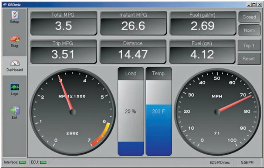
One of the many possible gauge setups from OBDwiz and TouchScan. The six gauges display fuel economy data with engine rpm, vehicle speed, engine load, and temperature. Courtesy ScanTool.net
