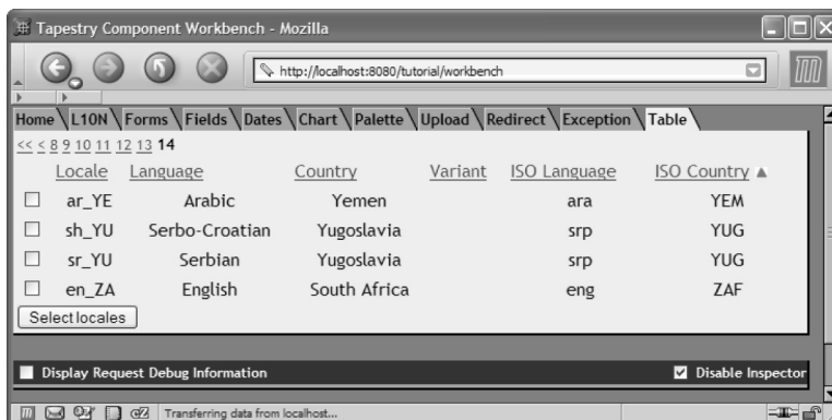
Figure 6.6 The Tapestry table component is quite powerful when customized. This example shows automatic paging, controls in columns, and sortable columns.
