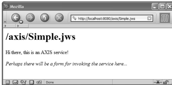
Figure 18.3 Accessing the web service via an HTTP GET displays a message indicating that a web service is running at that URI.
