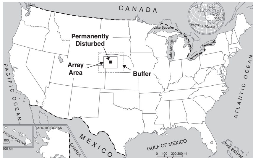
FIGURE 7.39 Estimated area required to meet half of U.S. electricity demand with wind turbines.
