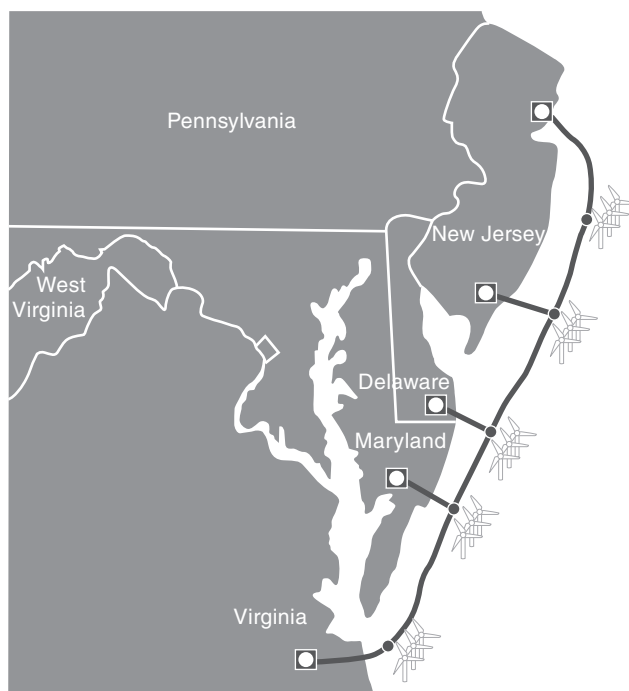
FIGURE 7.46 Proposed Atlantic Wind Connection transmission backbone for offshore wind farms.
