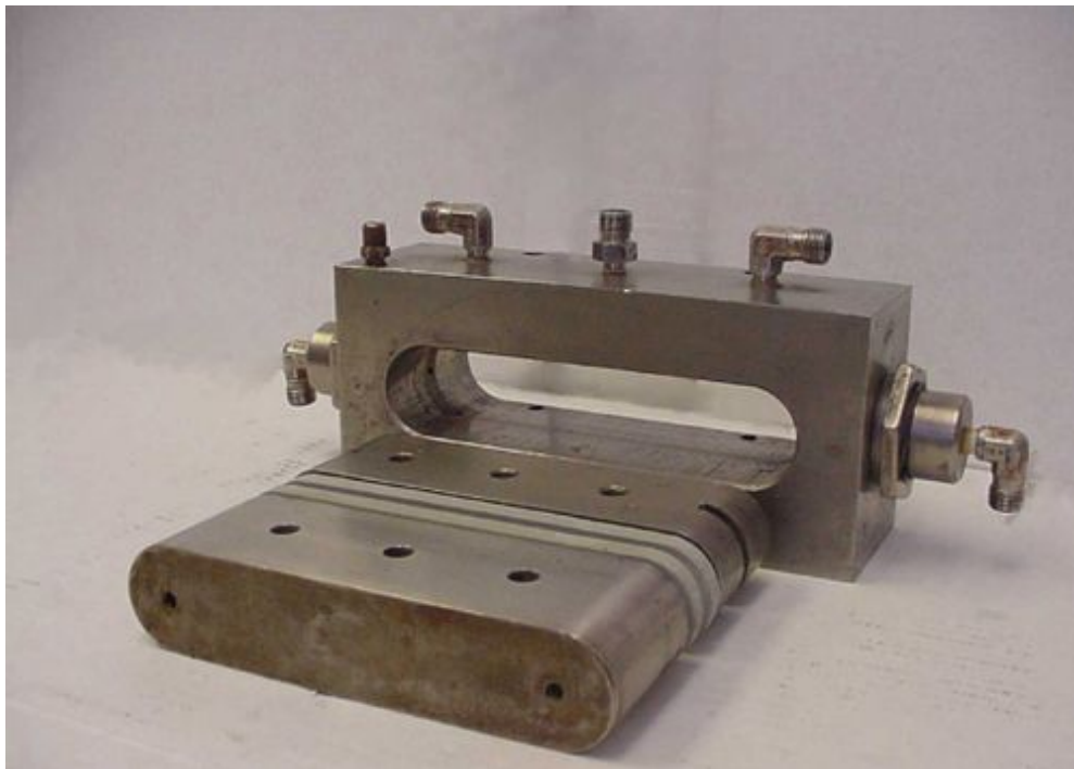
Figure 18-16. API Cell for the laboratory determination of proppant conductivity. (From Brannon, 2007 .)
