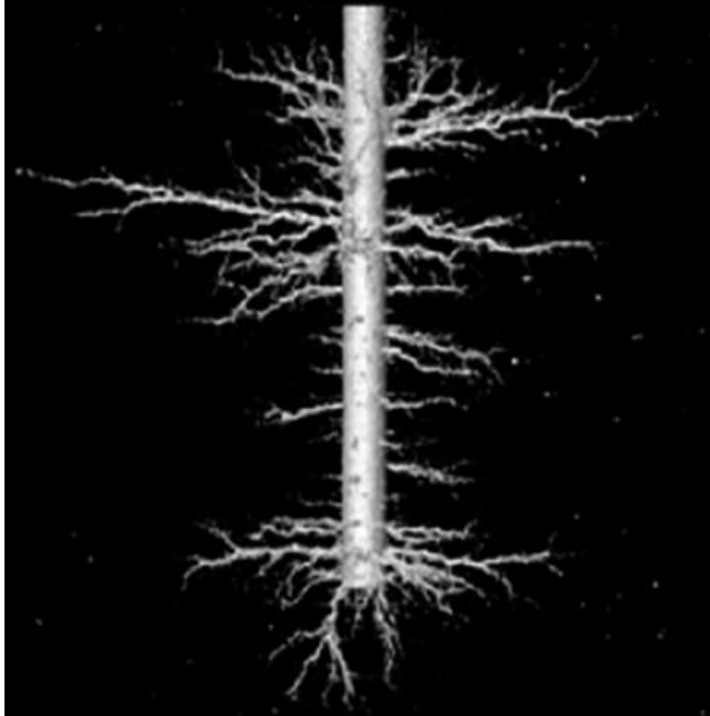
Figure 16-1. Wormholes created in a large block experiment. (From McDuff et al., 2010. )
