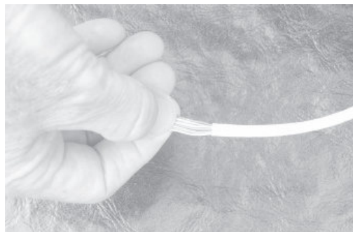
Figure 7-2 Flatten and arrange wires in the correct order.
