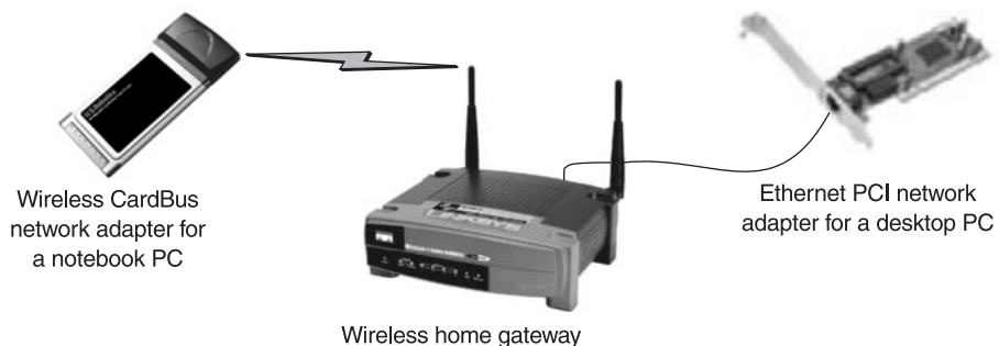
Figure I-5 In Chapter 5, you learn about the hardware that enables connectivity between PCs and other devices in a home network. A central hub, the home gateway, and the internal or external network adapters work together to permit wired and/or wireless links between PCs and network devices. The home gateway is a multifunction device that can serve as a router to bridge the home network to the Internet, a wireless access point (AP), and a switch for wired connections.
