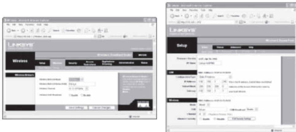
Figure 8-8 Basic wireless settings for a Linksys Wireless-G Broadband Router and a Linksys Wireless-G Access Point (at the bottom under Wireless)
