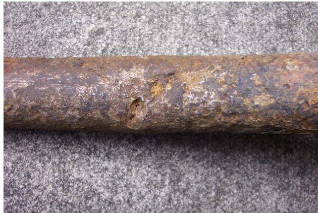
FIGURE 27.13 Pitting corrosion in an underground water pipe.
