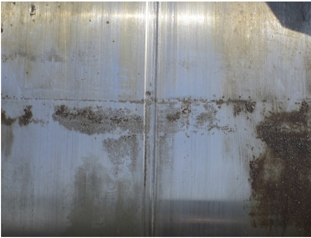
FIGURE 29.10 Abrasive wear track on crank-pin of marine diesel engine with a width of 8 mm and a depth of 0.2 mm.
