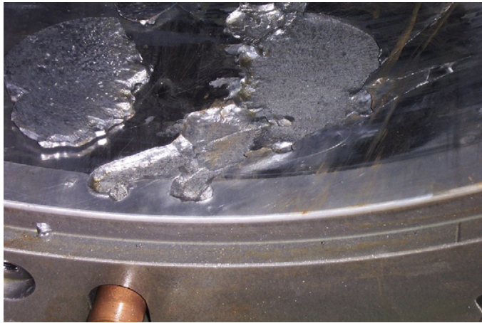
Propeller shaft white metal bearing
