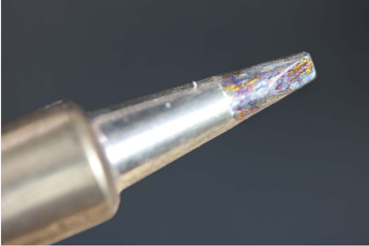
FIGURE 3-3: A dirty soldering iron
