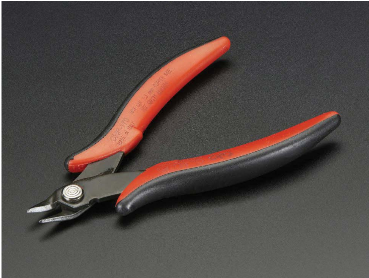
FIGURE 2-19: Diagonal flush cutting pliers are the best choice for hobby electronics. IMAGE COURTESY OF ADAFRUIT INDUSTRIES, CC BY-NC-SA 2.0.
