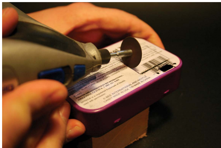
FIGURE 2-38: Cutting the holes. Be careful and wear safety glasses!
