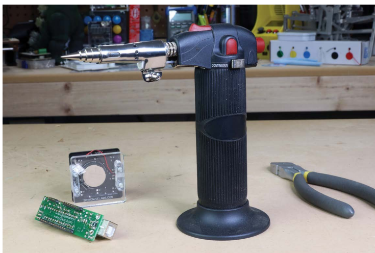
FIGURE 2-14: Gas-fueled soldering iron
