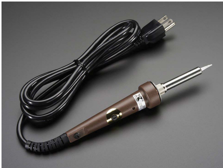
FIGURE 2-9: A 20 W, variable-temperature soldering iron IMAGE COURTESY OF ADAFRUIT INDUSTRIES, CC BY-NC-SA 2.0.
