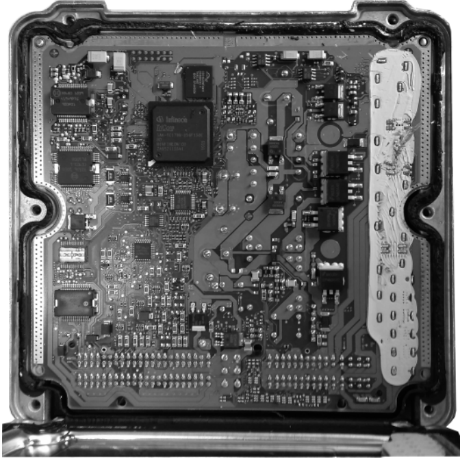
Figure 1.1 Board of an electronic engine control unit with heat conducting area on the right side
