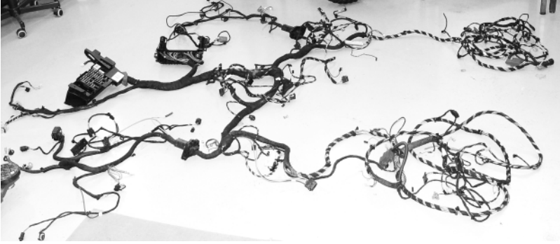
Figure 7.1 Engine cable harness with fuse box laid out on the floor
