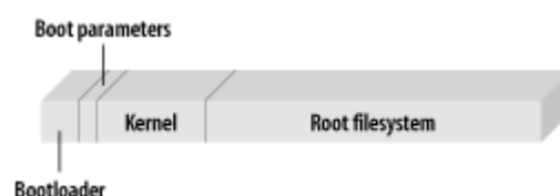
Figure 2-5. Typical solid state storage device layout
