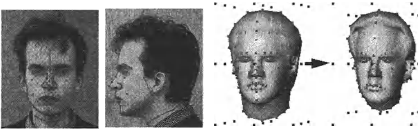
Photos and feature points The generic model An individual Fig. 1. Modification of a generic head according to feature points detected on pictures. Points on a 3D head are control points for DFFD.
