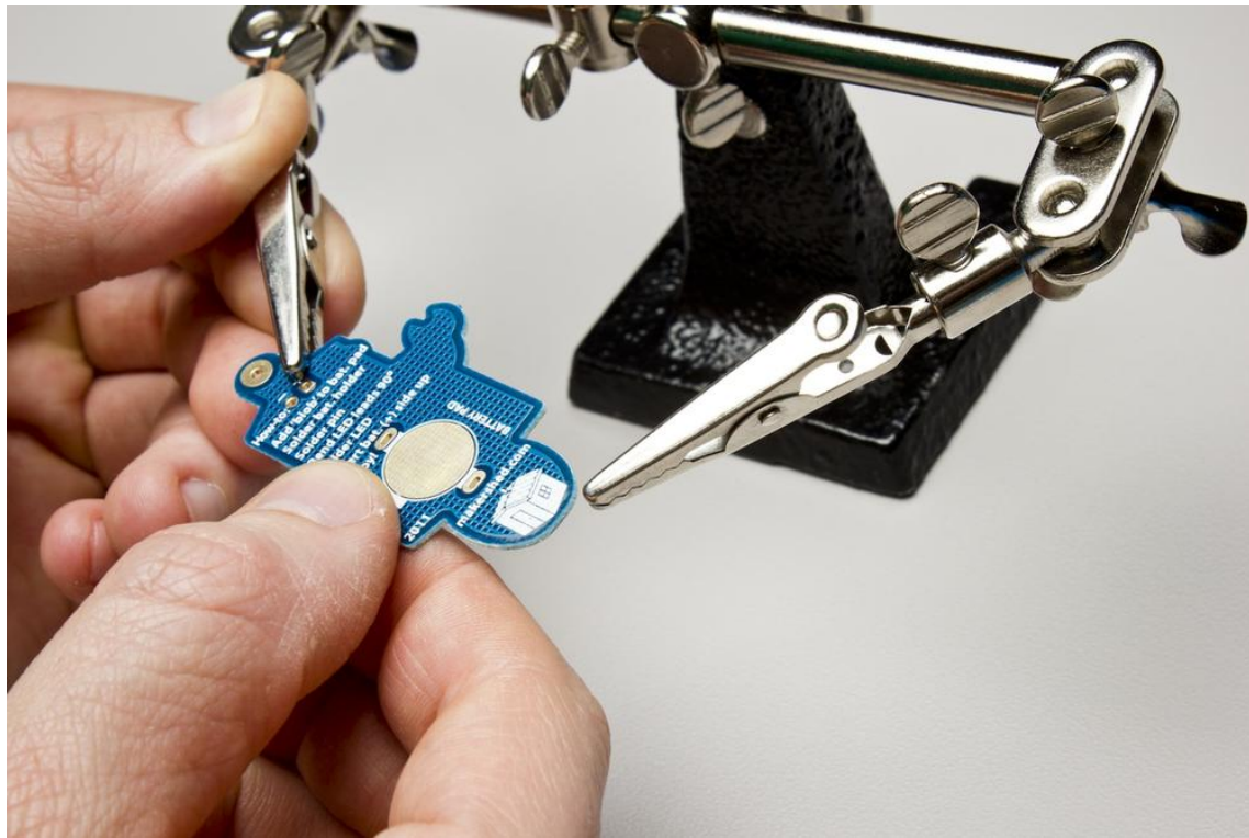
Figure 2-2. Holding a PCB in the helping hands
