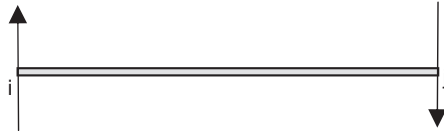
FIGURE 1.21. Positive shear forces.
