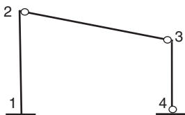
FIGURE 4.10. Results of calculations and plastic hinge location for stage 3.
