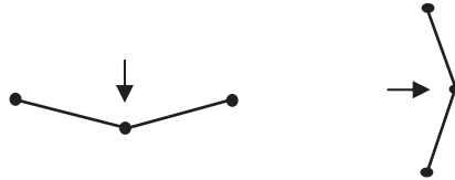
FIGURE 5.16. Beam mechanisms for beams and columns.
