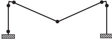
FIGURE 6.28. Feasible collapse mechanism.
