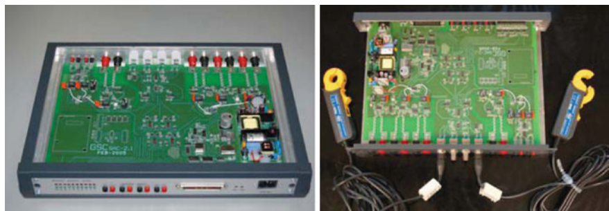
Fig. 8.5 Layout of the conditioning system, SAC-2
