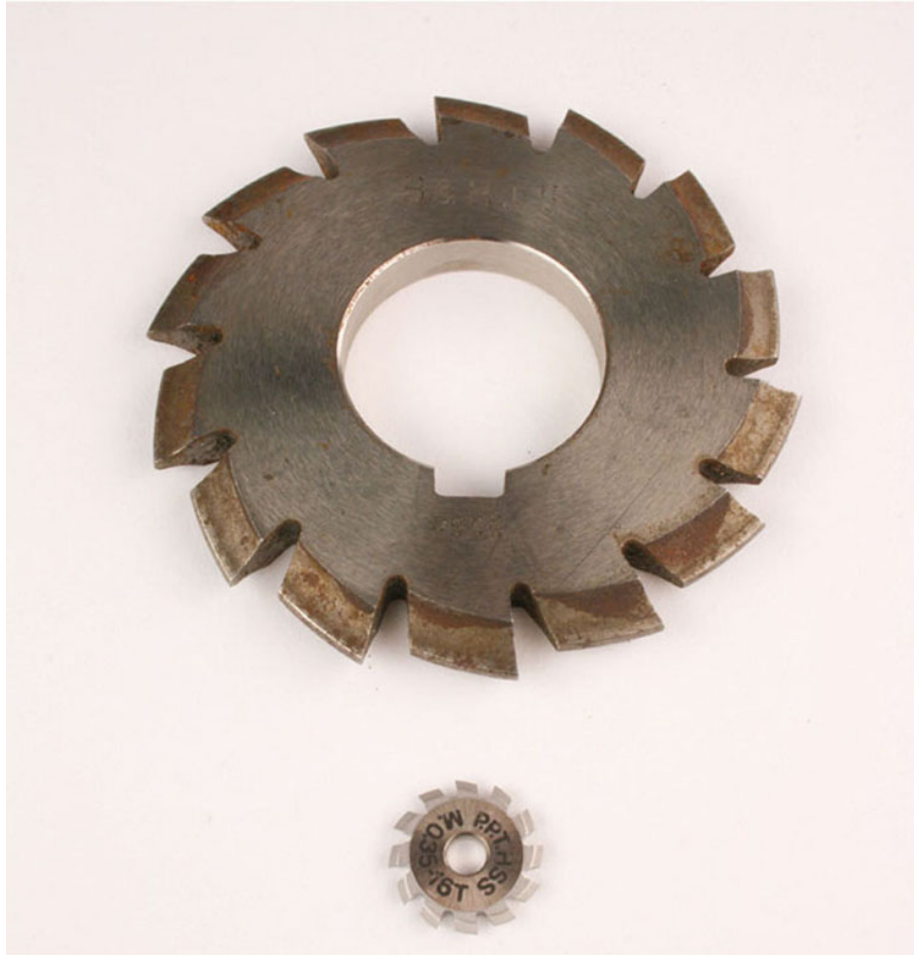
Fig. 4-21 Involute (upper) and cycloidal (lower) gear cutters.
