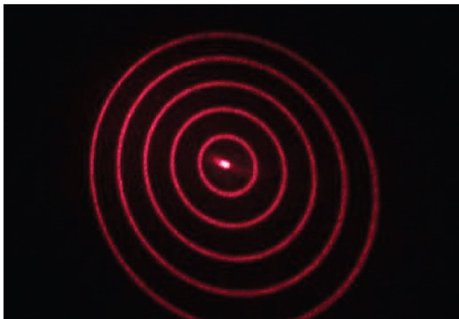
Fig. 2-24 A Laser Centre/Edge Finder fitted with a polarizing lens that projects a pattern of concentric
