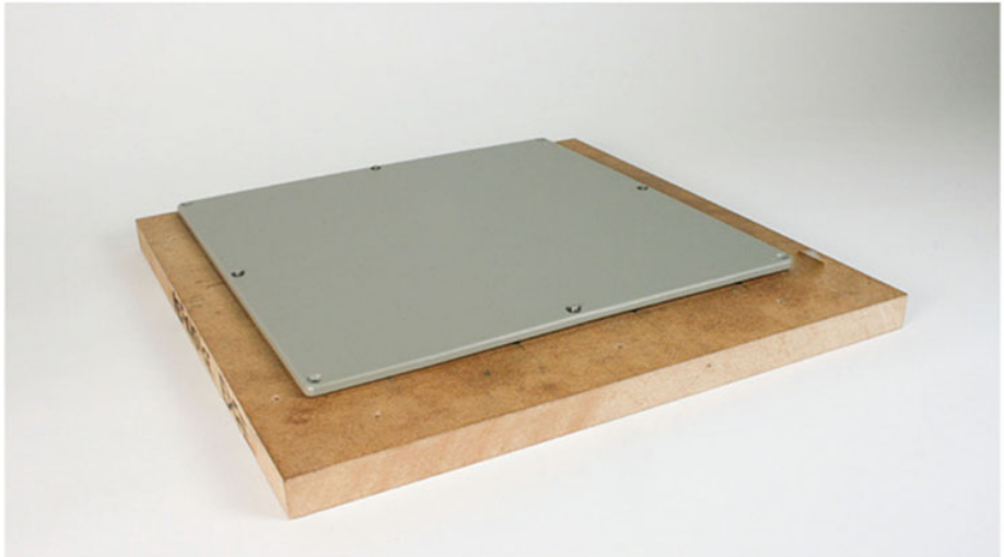
Fig. 7-15 Fixture showing the lid mounted in position for machining.
