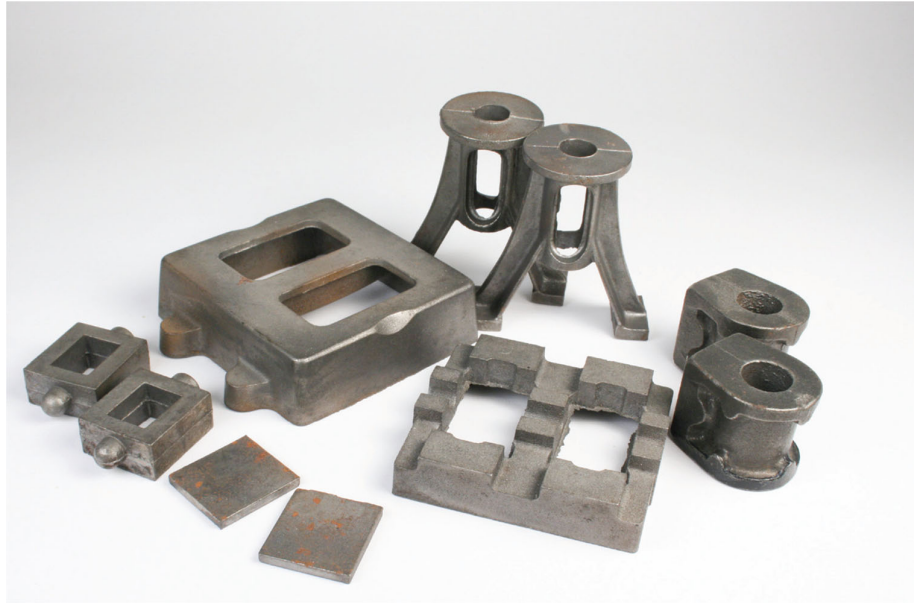
Fig. 8-4 Steam engine castings that could be mounted on a single fixture plate and machined as a batch.
