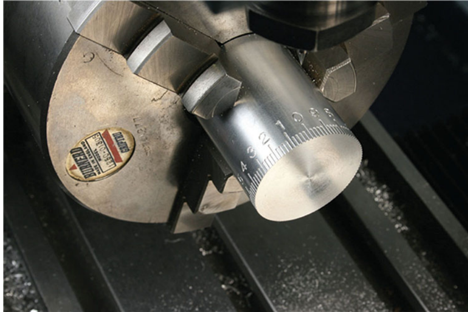
Fig. 10-19 An engraved scale comprising lines and numerals wrapped around a cylinder.
