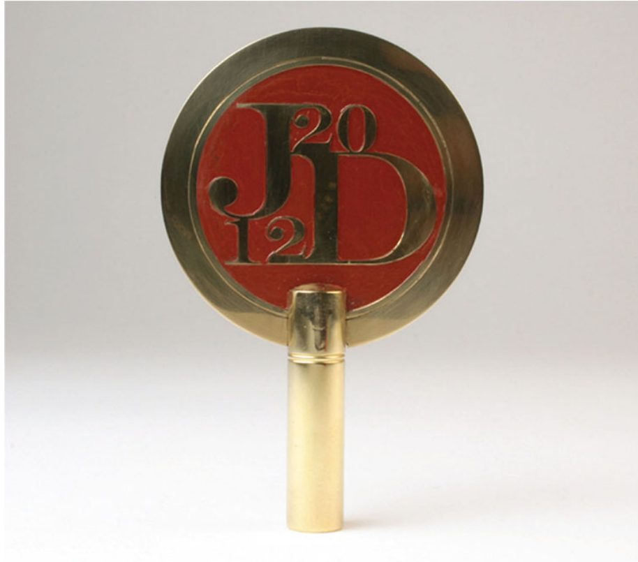
Fig. 10-17 Filling pockets with paint or another filler hides the tool marks and enhances the visual effect of an engraving.
