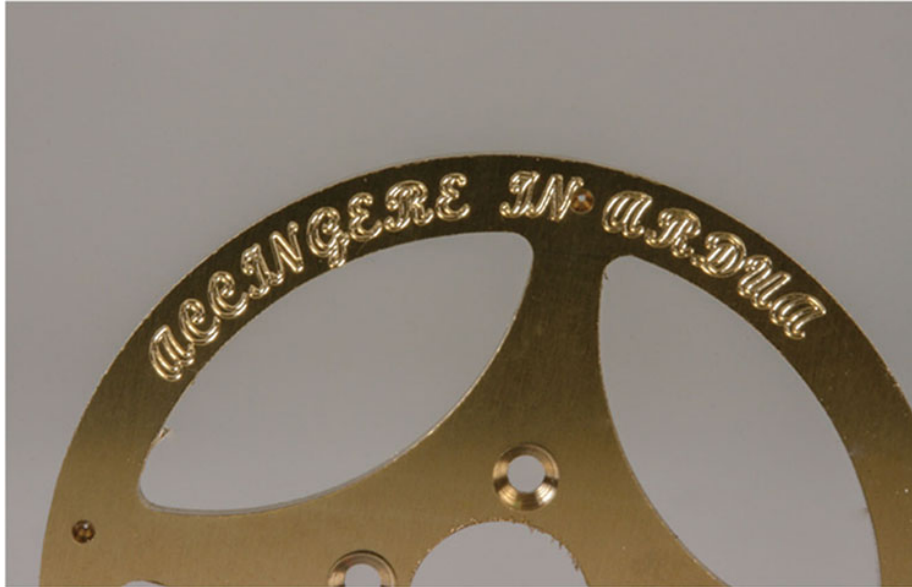
Fig. 10-5 Text engraved on a circular path around a clock wheel.
