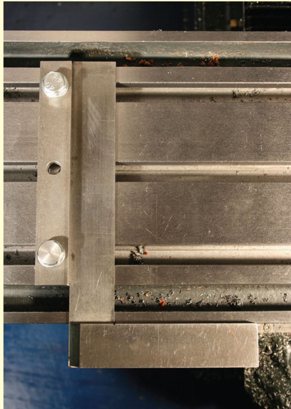
Fig. 5-6 Setting the stop bar across the table, using an engineer's square.
