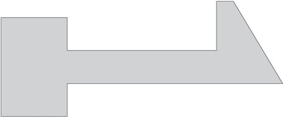
Fig. 6-11 A shape that would benefit from tabs to hold it in position.
