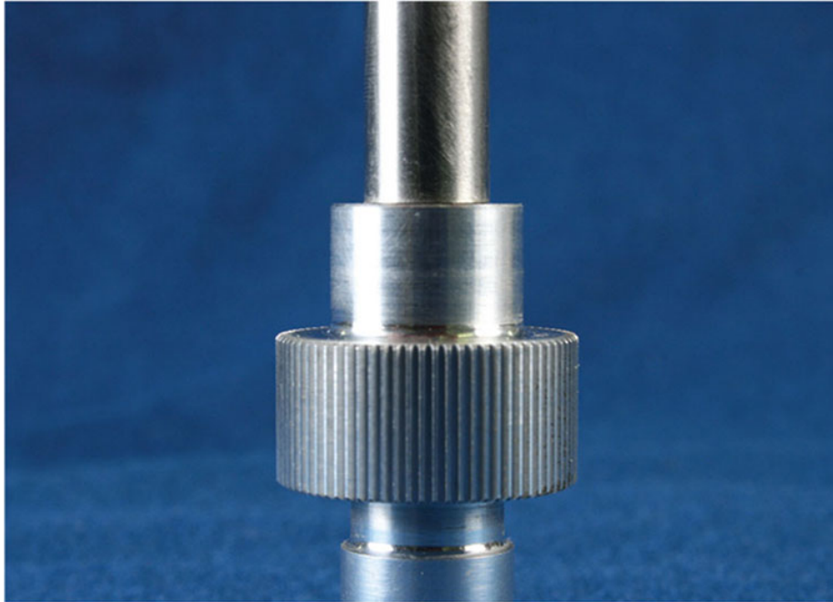
Fig. 10-20 Straight knurling can be created by engraving straight lines.
