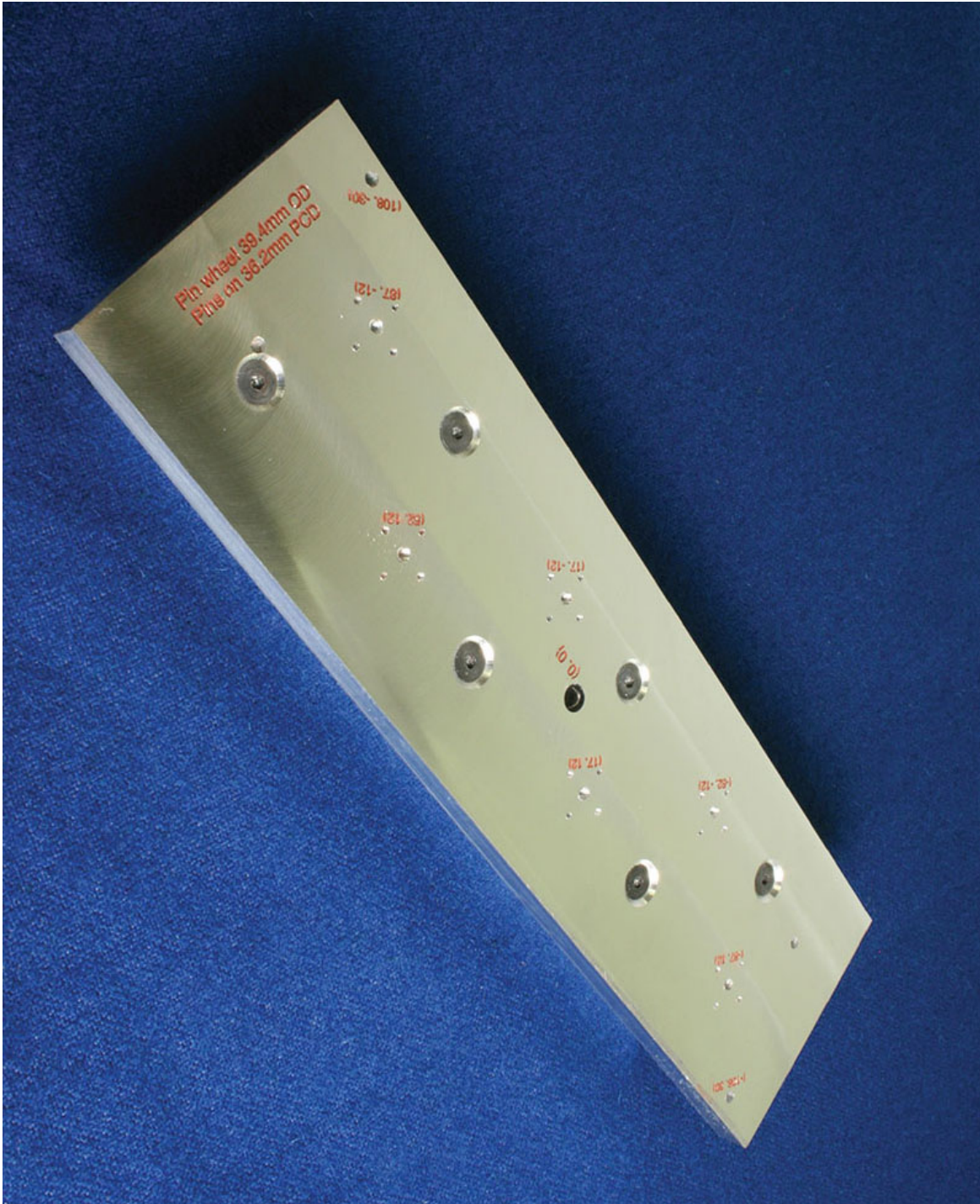
Multiple parts can be made using fixtures such as this one, which is used to make six clock wheels at a time.
