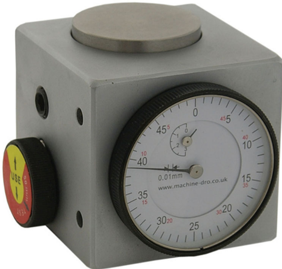
Fig. 2-30 An analogue Z height gauge based on a dial indicator. (Photo: Allendale Electronics)
