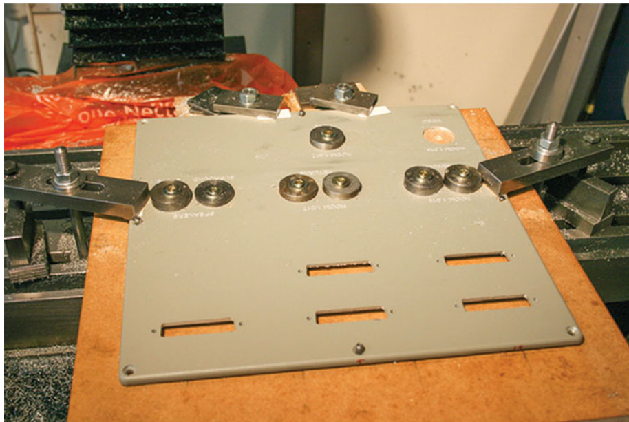
Fig. 10-7 Die-cast box lid pulled straight using large washers as clamps.
