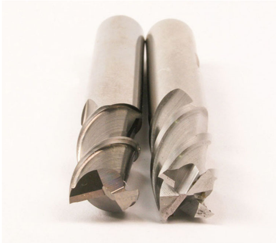
Fig. 4-12 A slot drill with two cutting edges and an end mill with four cutting edges.
