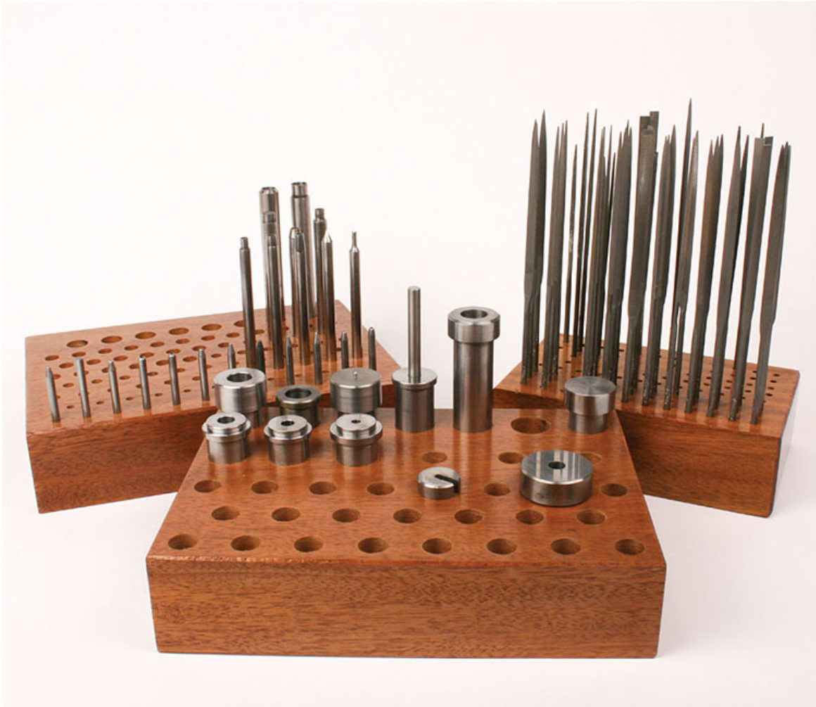
A selection of tool-holder blocks with patterns of holes that can easily be created using CNC drilling commands.
