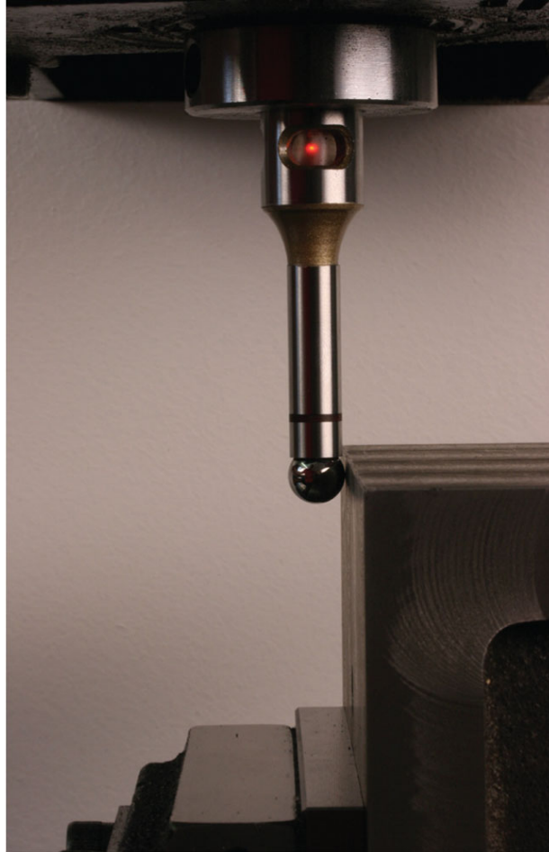
Fig. 2-14 An electronic edge finder indicating that it is in contact with the workpiece.
