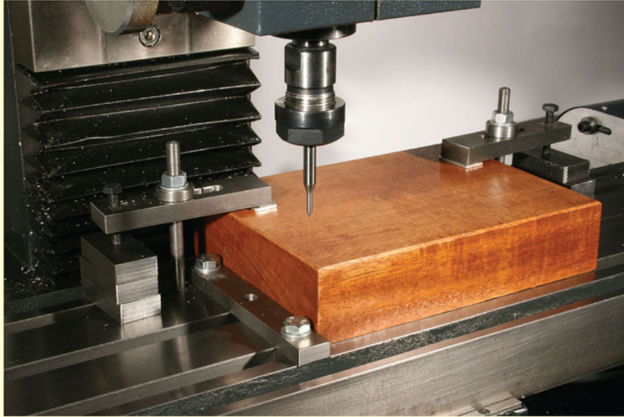
Fig. 5-11 The workpiece secured to the bed using clamps.
