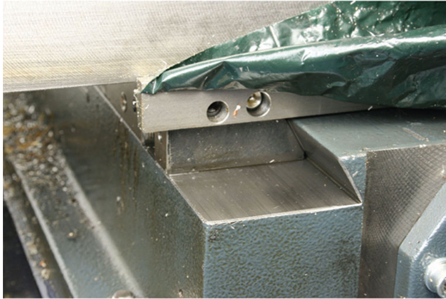
Fig. 1-14 A dovetail slideway on a cross slide.
