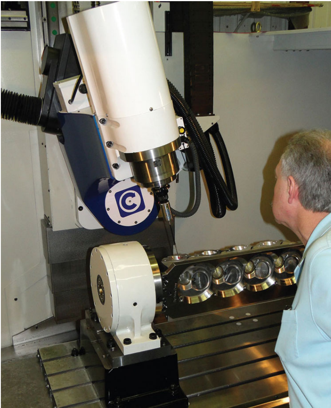
Finding the shape of holes in an engine block using a probe. (Photo: Centroid Corporation.)
