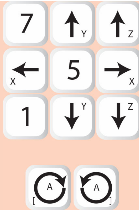
Fig. 3-4 Jog keys on the numeric keypad. The 'A' rotation keys may vary or be undefined.
