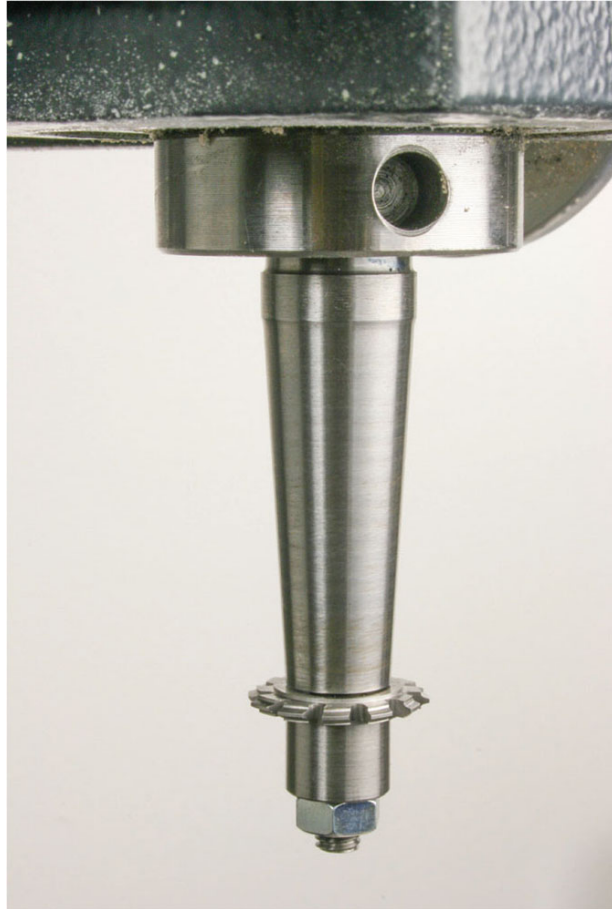
Fig. 4-22 A cycloidal cutter mounted on an arbor.
