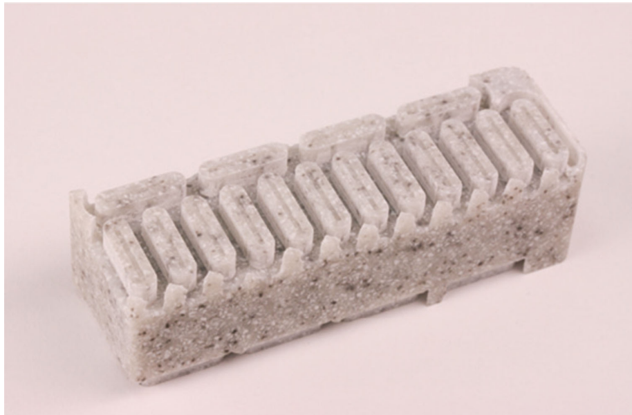
Fig. 8-2 Clock batons cut as a batch from the top and bottom faces of a single block of material, which acts as its own fixture.
