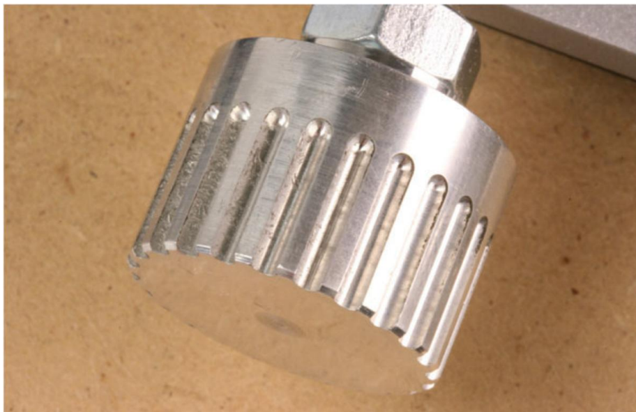
Fig. 10-21 Flutes can be created using a ball-nosed end mill.
