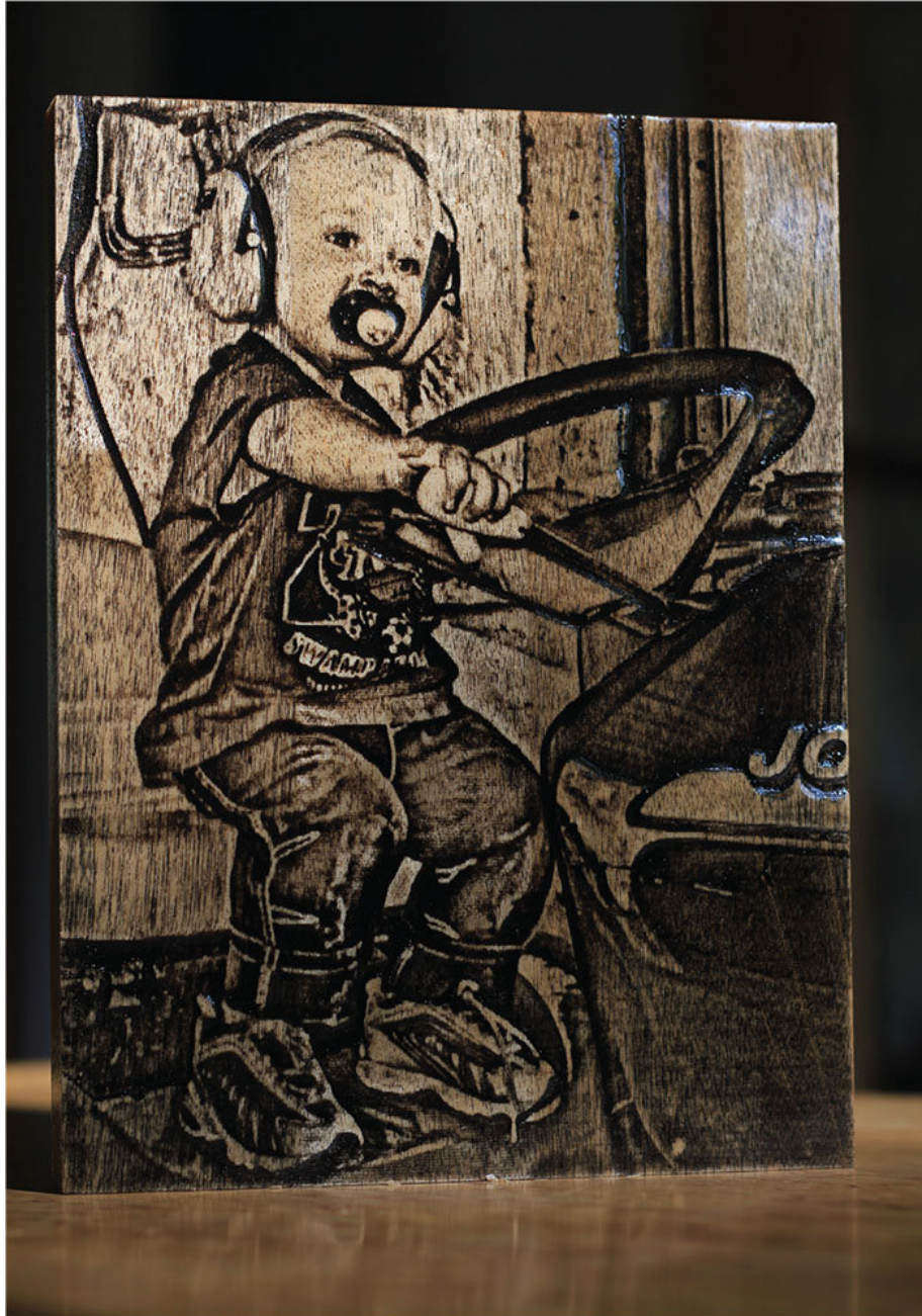
Fig. 10-33 Photoengraving produced from a photograph by using PhotoVCarve software. Photo courtesy of Markus Dahlberg at Pictures In Wood.
