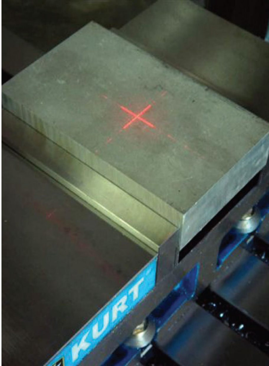
Fig. 2-22 Laser-generated cross hairs projected on to a workpiece. Note the length of the arms. (Photo: SDA Manufacturing)
