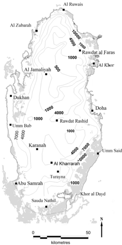
Figure 2.2 Salinity map of Qatar in 1980 in milligrams per liter total dissolved solids (TDS) (modified from Dastane and Al-Faihani 1980). The position of coastal sabkha are shown in gray.
