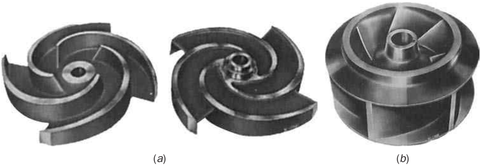
FIGURE 31.23 (a) Front and back views of an open impeller with partial shroud and pump-out vanes on back side. (b) Francis-vane radial double-suction closed impeller. (Source: Part (b) has been reprinted with permission from Flowserve Corporation.)
