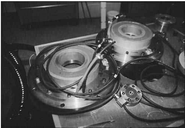
FIGURE 29.10 Axial magnetic bearing stator. (Source: Revolve Technologies, Calgary, Alberta, Canada.)
