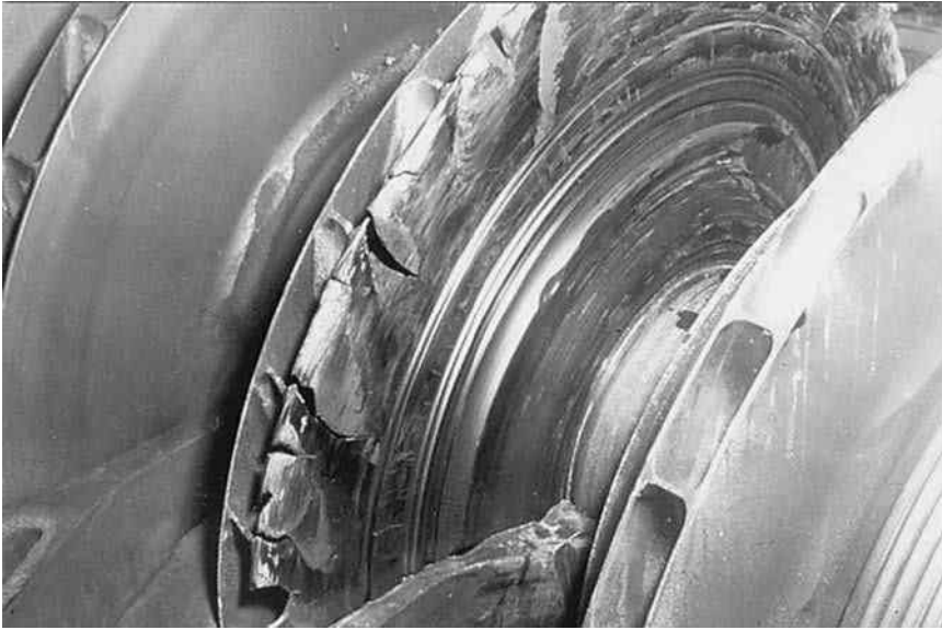
FIGURE 25.39 Damage caused by compressor surge.
