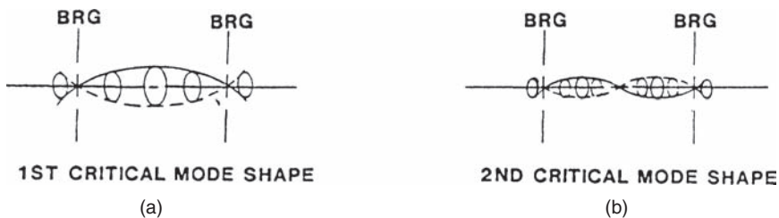
FIGURE 25.38 Rotor lateral critical speed mode shapes: (a) first critical mode shape, (b) second critical mode shape.
