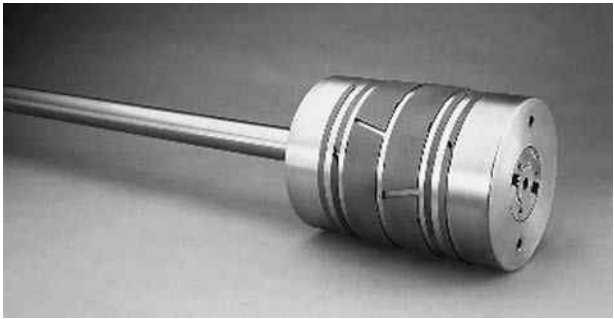
FIGURE 17.34 PTFE rider bands used to support pistons of contact-type non-lubricated compressors. (Source: Dresser-Rand Company, Painted Post, N.Y.)
