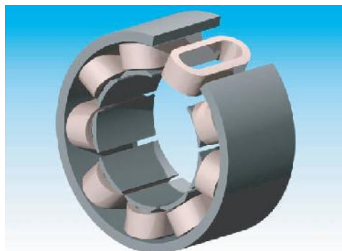
Figure 2. SMC stator. One SMC tooth missing. Design Alan Jack, Newcastle University.
