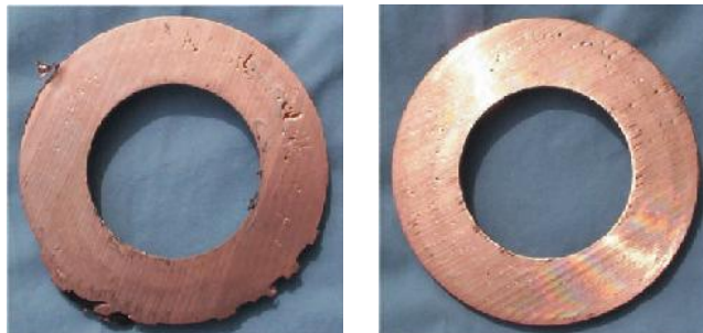
Figure 9. Photographs of sectioned end rings with 55% prefill. Ejector end ring on left; gate end ring on right.
