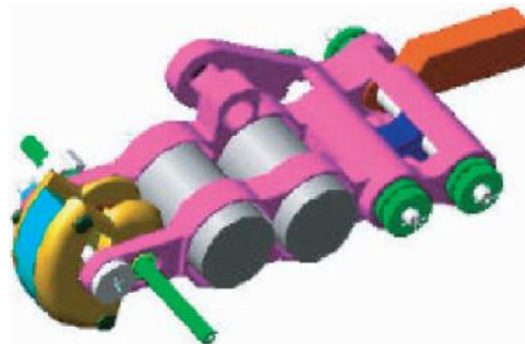
Figure 2. Hand prosthesis mechanism prototype driven by two rotating mode piezomotors [5].
