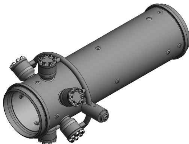
Figure 7.5 Radial discharge mechanically atomised attemperator. © SPX Flow, reproduced with permission
