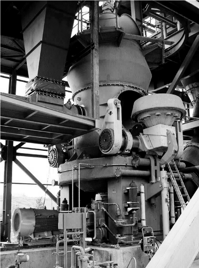
Figure 3.14 Roller retracted for maintenance. © Loesche, reproduced with permission
