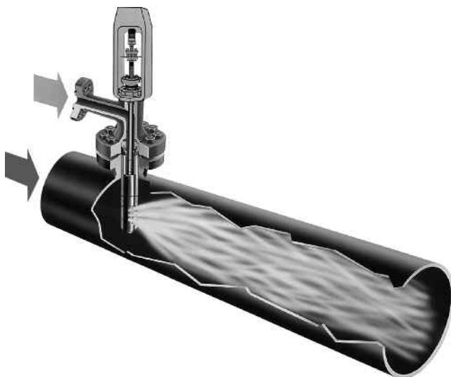
Figure 7.2 Principle of a multinozzle desuperheater. © SPX Flow, reproduced with permission
