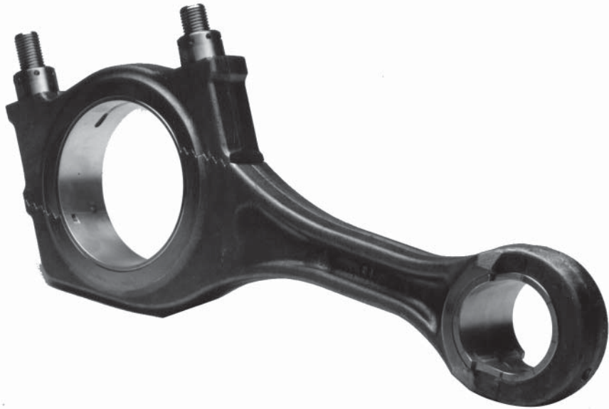
Figure 27.13 The connecting rod of the Wärtsilä 20 engine incorporates a stepped split
