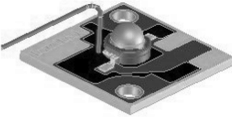
Figure 11.5 Location of Thermocouple to Measure LED Temperature.
