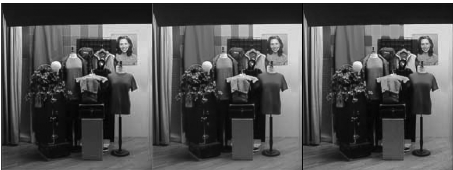
Figure 3.13 Left: Cool White Fluorescent 4100 K, CRI 60; Middle: Incandescent, 2800 K, CRI 100; Right: Reveal® Incandescent 2800 K, CRI 78.
