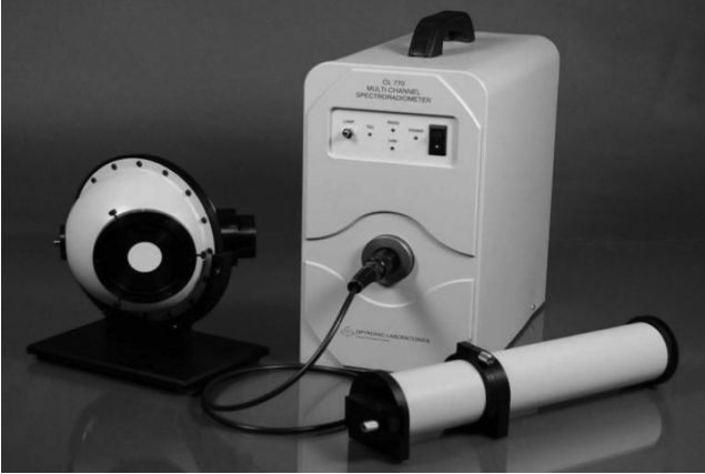
Figure 11.4 Gooch & Housego 6-Inch Integrating Sphere with OL770-LED Spectroradiometer. Source: http://www.olinet.com//content/file/1210967318B220_770-LED_Brochure.pdf .
