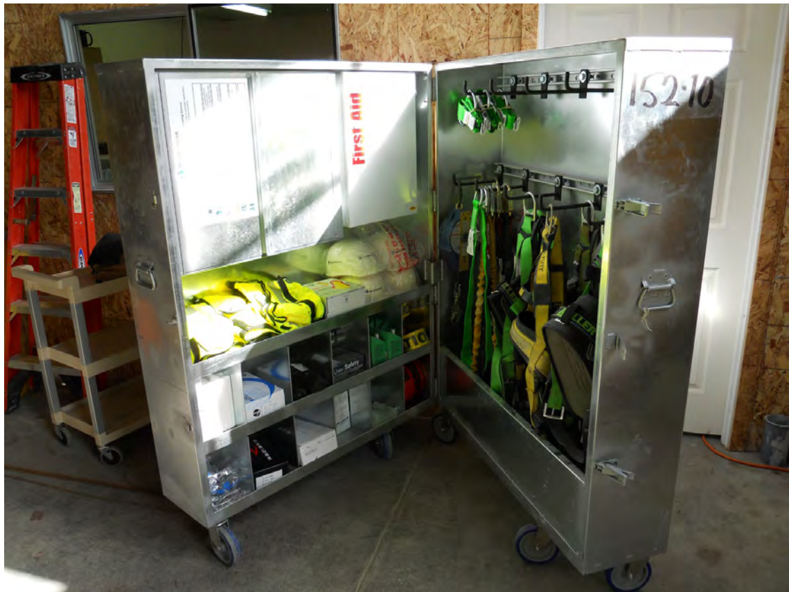
Figure 9-3 Example of Safety PPE Cabinet (Picture Courtesy of Korsmo Construction)
