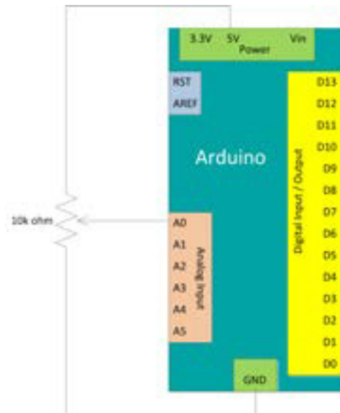
Figure 9-6. Schematic diagram of potentiometer connected to Arduino™ Uno
