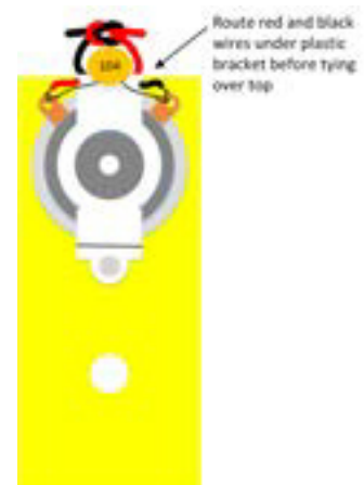
Figure 14-6. Wire routing on DC motor with square knot
