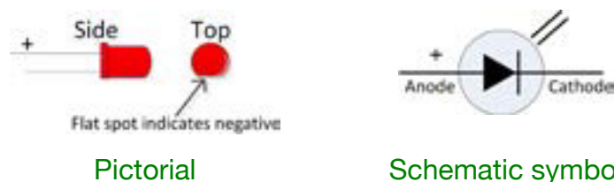
Figure 4-2. LED shown in pictorial and schematic forms
