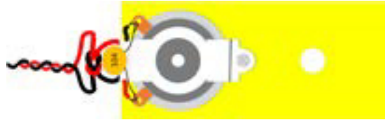
Figure 14-7. Twisted wire routing on DC motor
