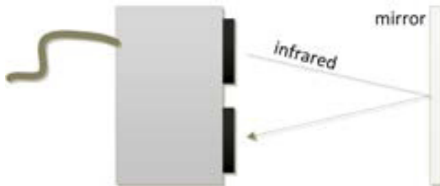
Figure 13-1. Garage door obstacle detectors
